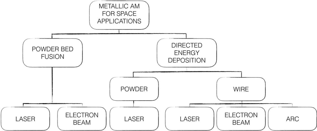
**Figure 1. Overview of additive manufacturing methods for space applications**
