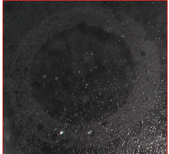
*Fig. 2 Snow-blasted ice surface pictured after a friction test with a rubber ring.*
