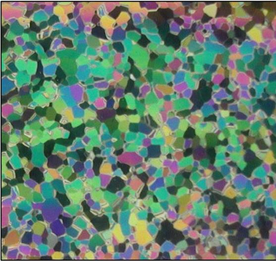
*Fig. 1 Horizontal thin section of the ice showing the size distribution. The average crystal diameter was about 2 mm.*
