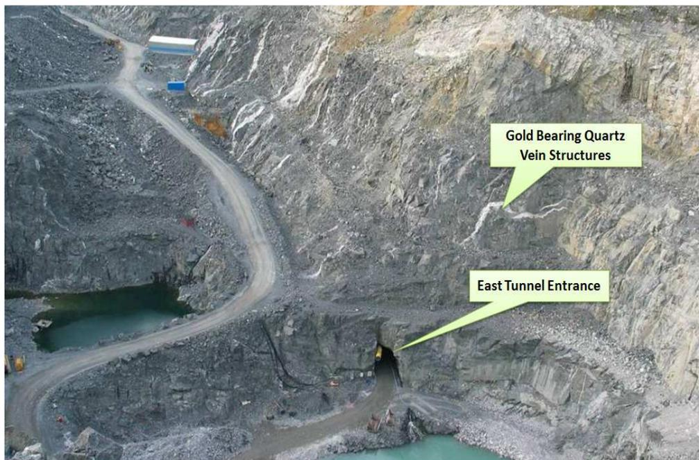
**Figure 4 View of gold bearing quartz veins and main tunnel from open pit (www.goldore.ca)**
