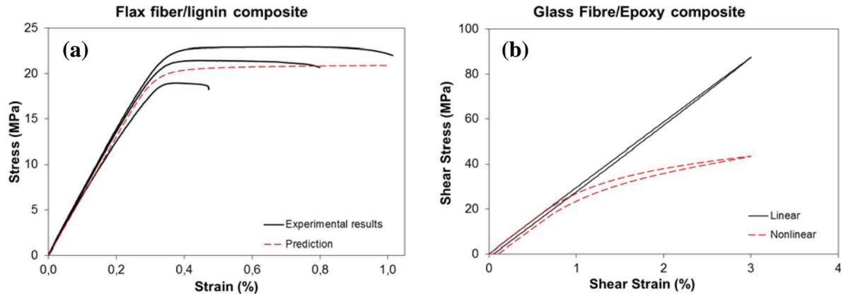
Figure 1: Simulated and experimental tensile stress-strain curves in strain controlled test for (a) standard loading ramp for flax fibre/lignin composite and (b) slow loading-unloading ramp for Glass fibre/epoxy  $[\pm 45]_S$  composite using linear and non-linear viscoelastic models
