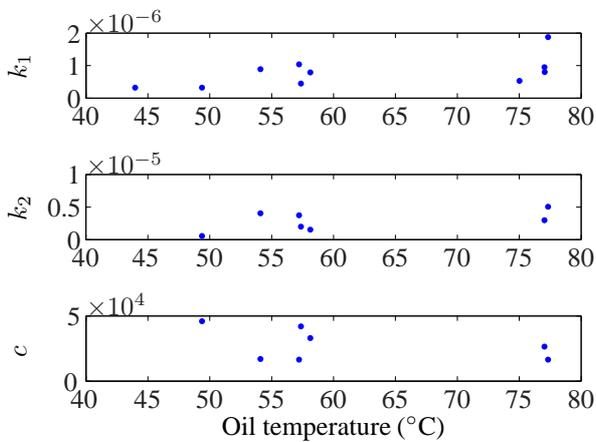
Figure 4: Wear coefficients plotted against lubricant temperature
