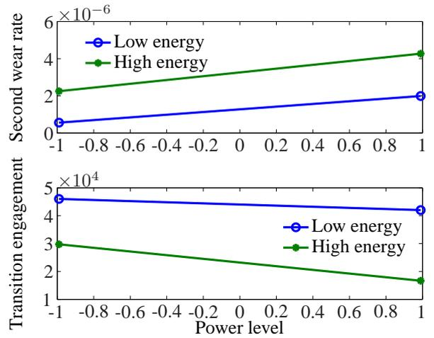
Figure 5: Interaction plot for power and energy with regards to second wear rate and wear rate change
