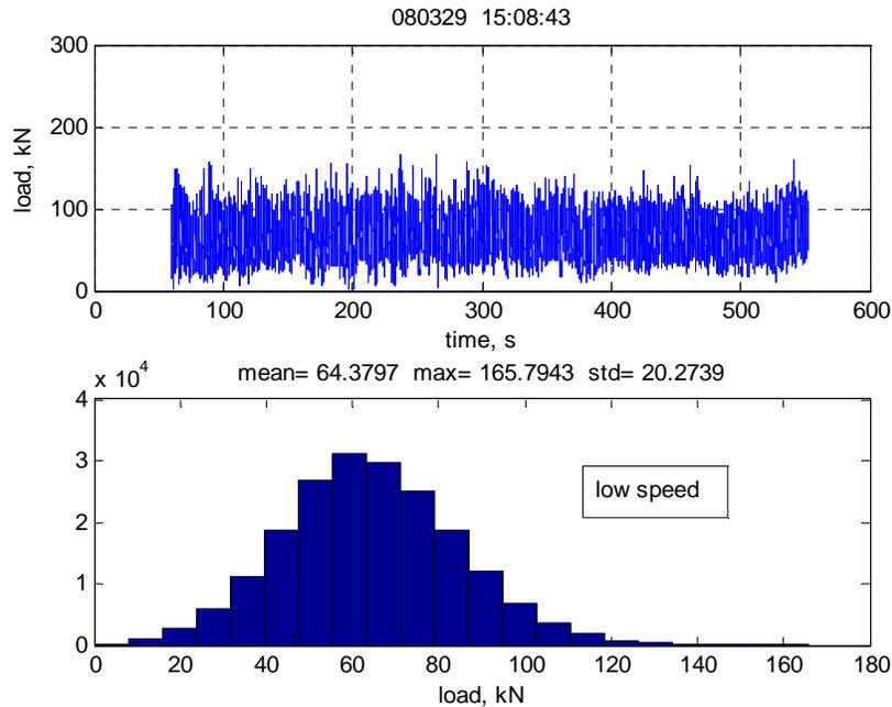
Figure 6. Ice load record from ice crushing tests number 12.
