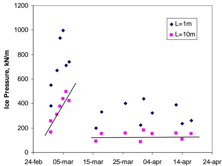
Figure 2. Seasonal variations of the empirically calculated maximum ice pressures on 1 m contact width (blue) and on 10 m (red with a line).
