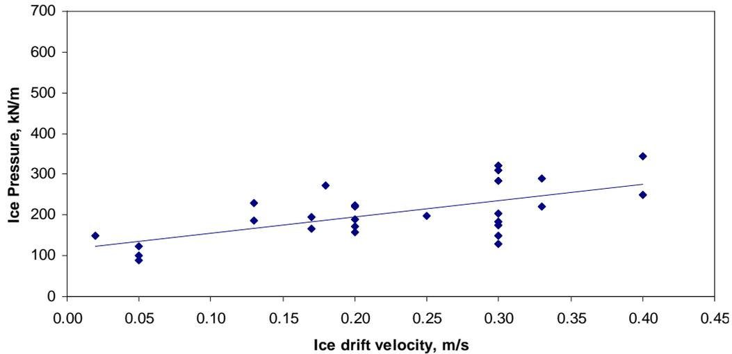
Figure 4. Obtained velocity effect on measured ice pressures winter 2000. Obtained pressures at zero velocity have been omitted (LOLEIF database, 2008).
