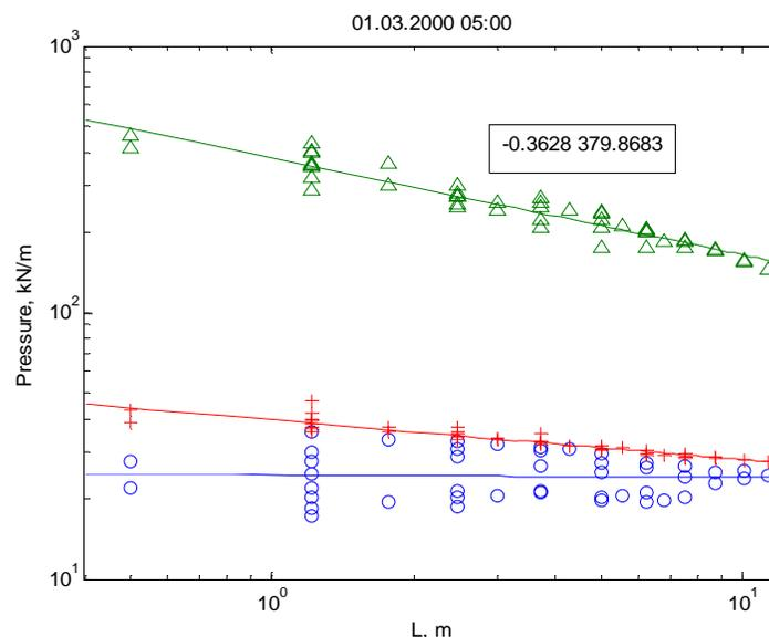
Figure 1. Example of analysed ice crushing event, where 8 panels were sustained to ice pressure. Max pressure (triangle), Standard deviation (+), average pressure (o).
