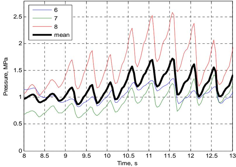
Figure 3. Oscillating ice pressures on three load panels at Lighthouse Norströmsgrund, April 10, 1999. Ice thickness = 0.7 m. (Fransson & Lundqvist, 2006).
