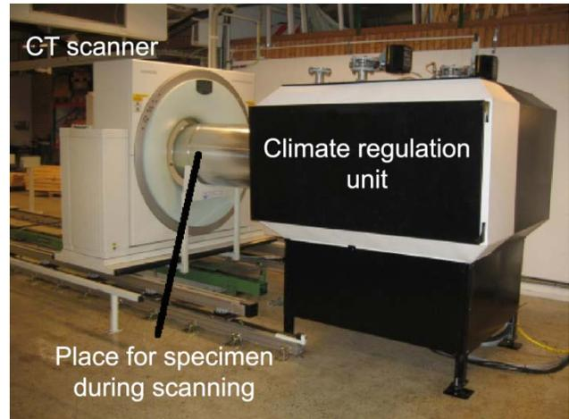
**Figure 3:** X-ray computed tomography (CT) with the climate chamber installed for CT measurements.
