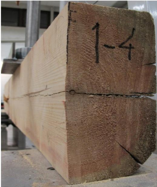
**Figure 2:** The beam of Scots pine used for crack analysis with the help of CT scanning.
