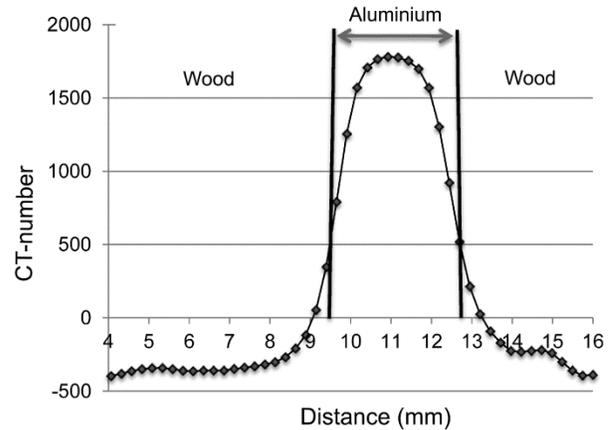
**Figure 12:** CT-number ( $CT_{MC}$  in Equation 2) showing moisture content variations in the wood-aluminium-wood direction of the specimen shown in Figure 11b
