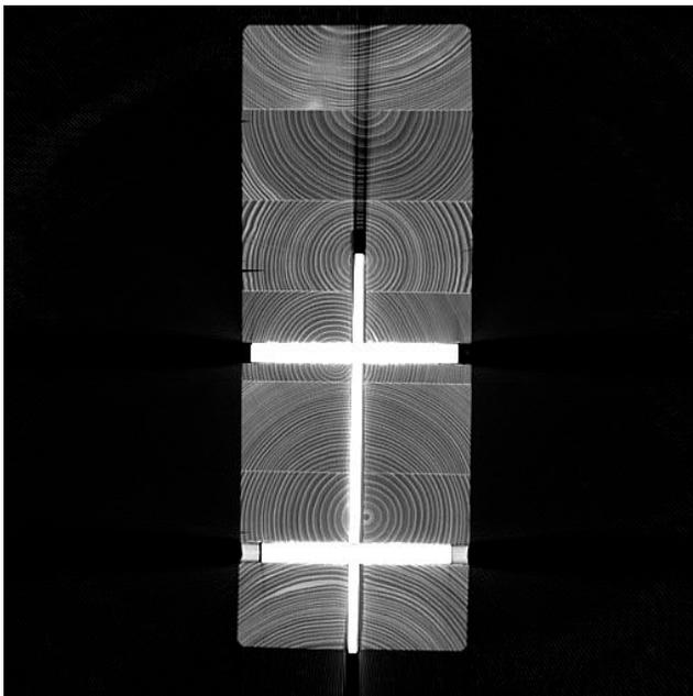
**Figure 9:** Cross-sectional view of a glulam beam of Norway spruce with an aluminium plate anchored with two aluminium dowels. The lower dowel is sealed with a silicon sealant. In the cross section, aluminium can be seen as white areas
