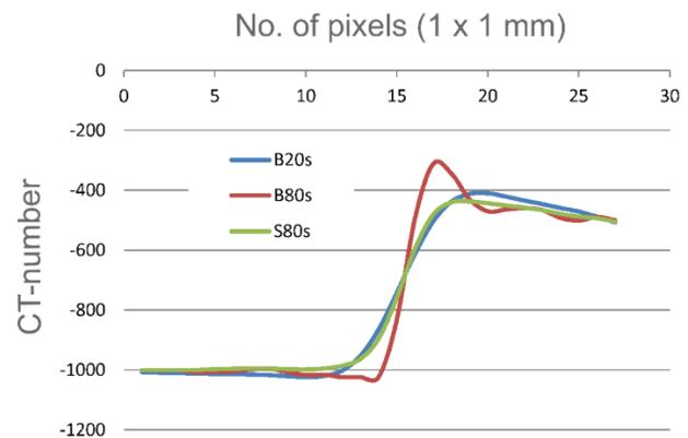
**Figure 8:** Detection of the edge of a wood specimen in CT-scanning using different reconstruction algorithms
