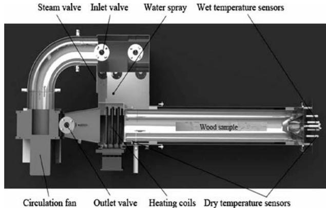
**Figure 5:** Exploded drawing of the climate chamber.
