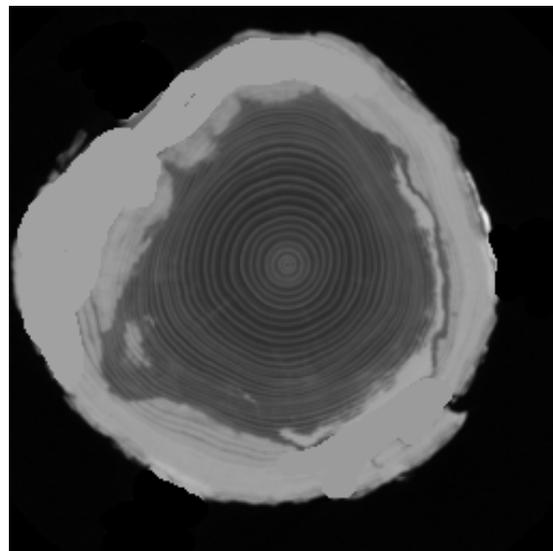
**Figure 4:** A cross-sectional image of a Scots pine log in which the densities at different positions in the object are shown in grey-scale form. High-density wood (wet sapwood) appears light in a CT image, while the dry heartwood appears darker grey.
