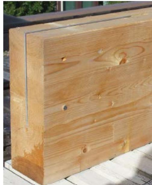
**Figure 1:** Glulam beam with aluminium plate and dowel. The distance from the end grain of the first couple of dowels was 50 mm. The next pair of dowels was 150 mm from the cross-section surface.
