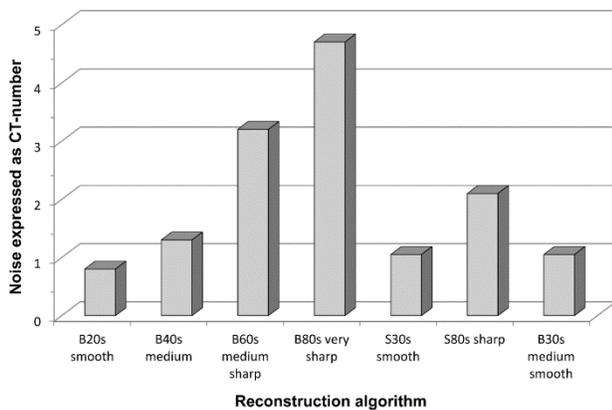
**Figure 6:** Measurement noise expressed as CT-number for different reconstruction algorithms in CT-scanner. Algorithms specified with a capital S at the beginning (e.g. S80s) are Shepps reconstruction algorithms
