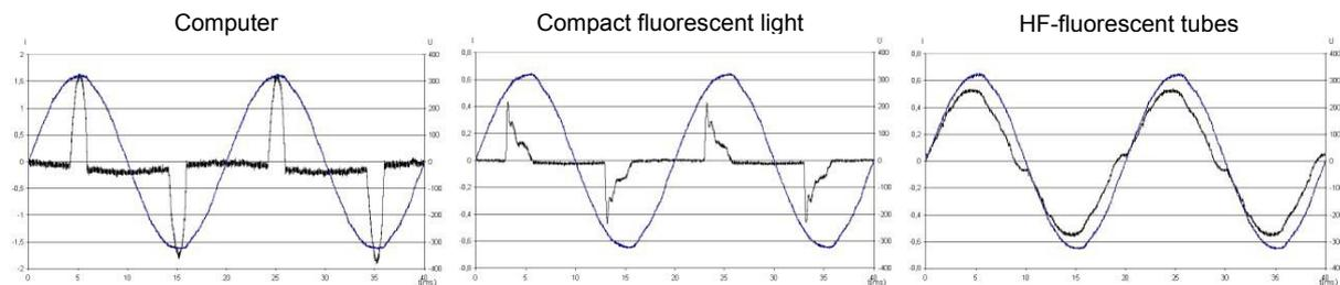
Figure 1 shows a few different electronic loads.
