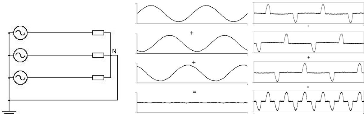
Figure 2 The current summation in the neutral point (left) for linear load (center) and non-linear load (right).
