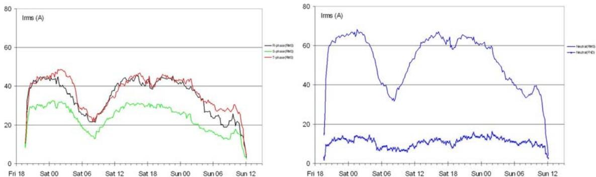
Figure 3 Variation of the phase-current (left) and neutral-current (right) during the weekend. The left-hand figure shows the rms current in the three phase conductors. The right-hand figure shows the rms value (top curve) and the fundamental value (bottom curve) of the neutral current.
