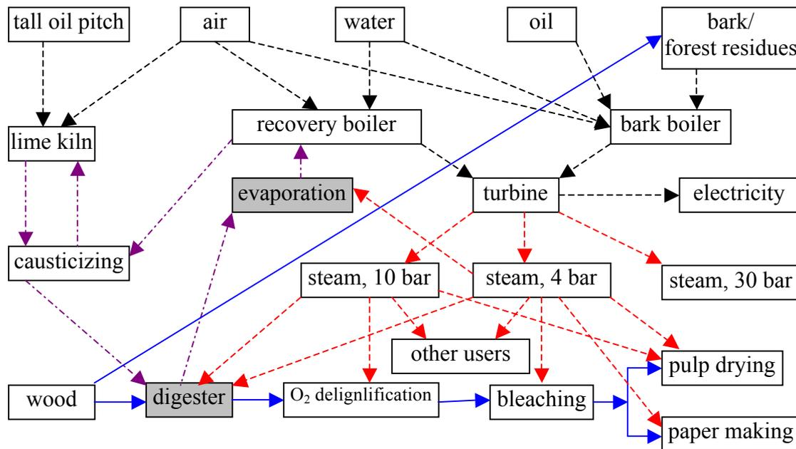
**Figure 1: Schematic description of the pulp and paper mill**
