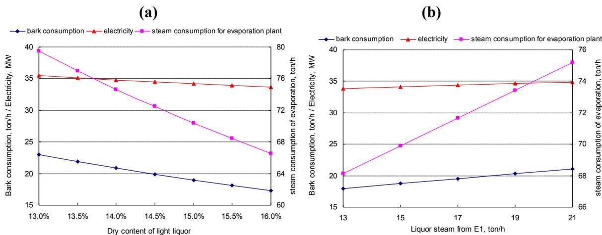
**Figure 7: The effect of the dry content of the light liquor (a) / the steam liquor to stripping (b) on the steam consumption of the evaporation plant and the performance of BB**
