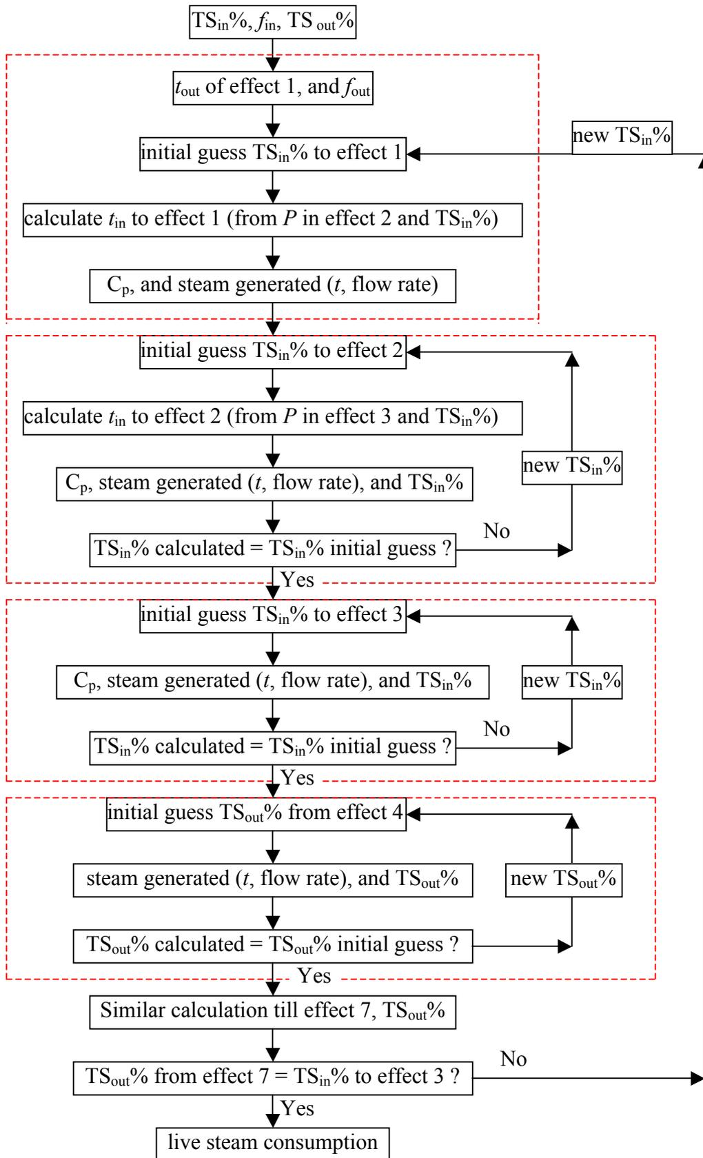
**Figure 3: Schematic illustration of the calculation for evaporation plant in Excel model**
