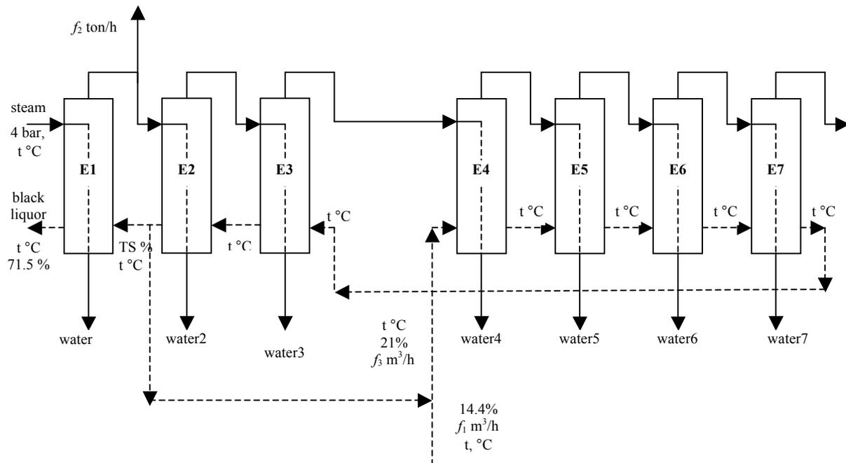
**Figure 2: Schematic description of the evaporation plant**
