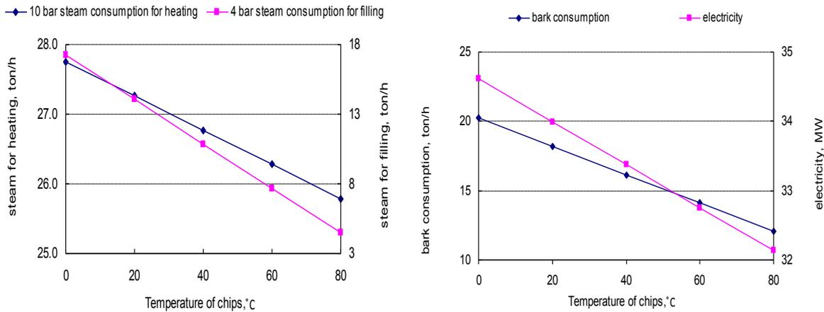
**Figure 8: The effect of the temperature of wood-chips on the steam consumption of digester and performance of BB**
