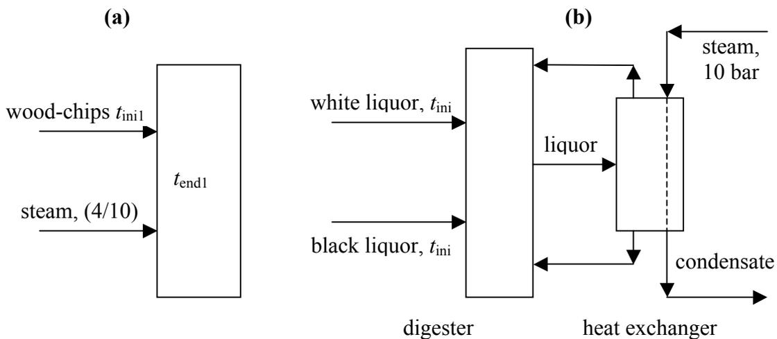
**Figure 5: Schematic representation of steps of filling and steaming (a) and steps of liquor filling and heating (b) for the digester**
