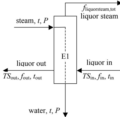
**Figure 4: Schematic representation of the effect 1 in the evaporation plant**
