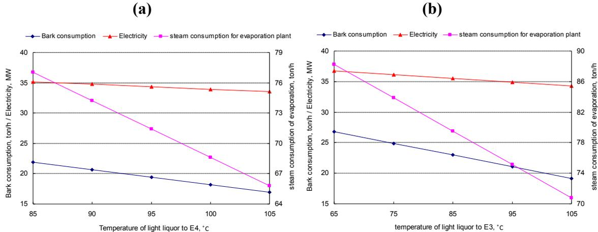
**Figure 6: The effect of the temperature of liquor to E4 (a) / the liquor temperature to E3 (b) on the steam consumption of the evaporation plant and the performance of BB**
