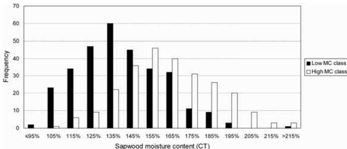
**Figure 4:** Observed sapwood moisture content (value from CT images) for 553 Scots pine sawlogs, separated into two classes depending on the sapwood moisture content predicted from simulated X-ray and 3D log scanner data.
