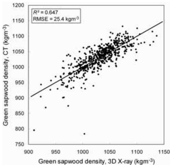
**Figure 1:** Sapwood green density in 560 Scots pine sawlogs, measurements in CT images versus predictions from simulated X-ray and 3D log scanner data.
