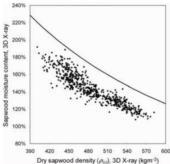
**Figure 5:** Estimated moisture content as a function of the estimated dry density in the sapwood of 553 Scots pine sawlogs. The solid line represents the theoretical maximum moisture content of saturated wood.
