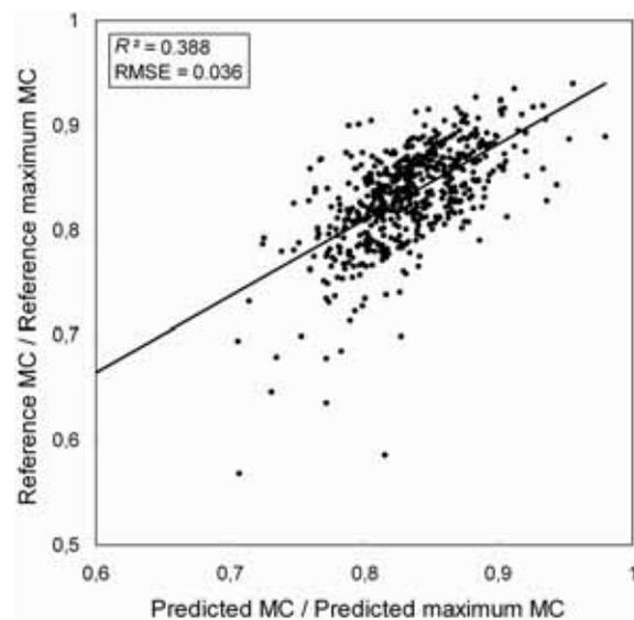
**Figure 6:** Sapwood moisture content relative to the theoretical maximum moisture content of saturated wood, measurements in CT images versus predictions from simulated X-ray and 3D log scanner data for 553 Scots pine sawlogs.
