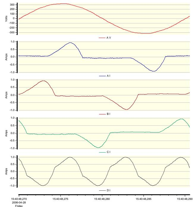
Figure 5. Measurements made on three computers connected to three phases. The two top graphs showing a phase voltage and the corresponding phase current, next the two remaining phase currents and the neutral current.
