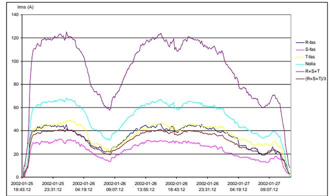
Figure 1. The three phase and the neutral currents during LAN 2002
