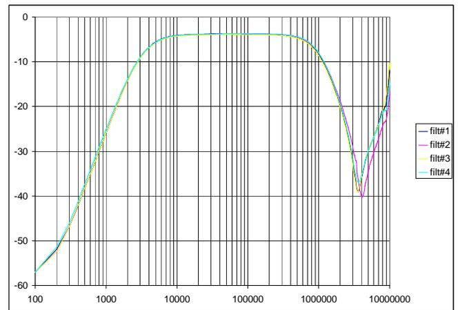
Figure 8. Frequency response in filter used for voltage measurements. The amplitude loss in the pass band is 4 dB
