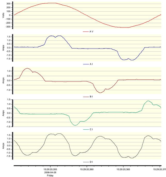
Figure 6. Measurements made on three LCD:s and three computers together connected to three phases. The two top graphs showing a phase voltage and the corresponding phase current, next the two remaining phase currents and the neutral current.
