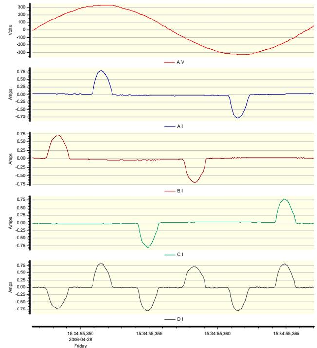
Figure 4. Measurements made on three LCD:s connected to three phases. The two top graphs showing a phase voltage and the corresponding phase current, next the two remaining phase currents and the neutral current.
