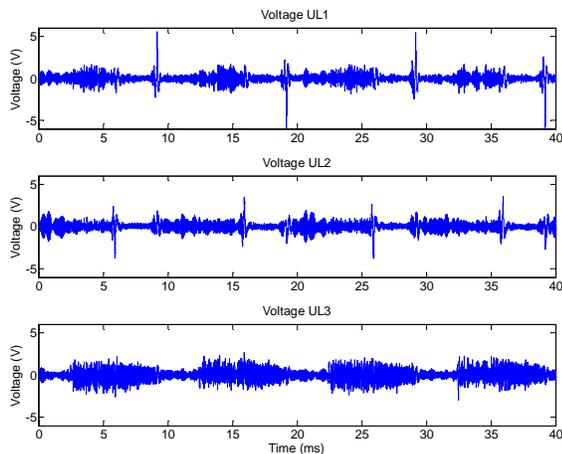
Figure 7. Measurements made on three phases of fluorescent lamps. Phase L1 (on top) has 55 fittings connected, phase L2 (in the mid) has 56 fittings connected and phase L3 (at the bottom) has 9 fittings connected.
