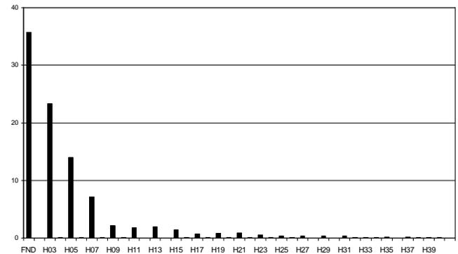
Figure 2. The phase currents harmonics during LAN 2002
