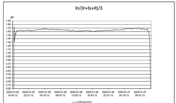
Figure 3. The three phase and the neutral currents during LAN 2002
