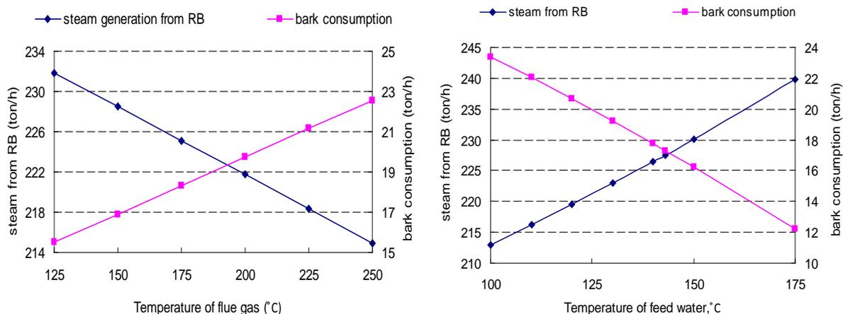
Fig.3. The effects of temperature of flue gas and feed water on the performance of the RB and the BB.
