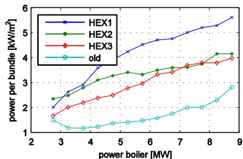
**Figure 6:** Heat transfer in the condensing heat exchanger before and after the installation.
