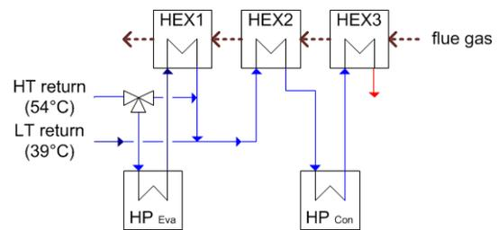
**Figure 4:** Sketch of the active condensation system: Condensing heat exchanger with heat pump.
