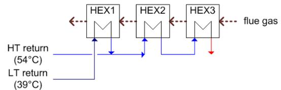
**Figure 3:** Sketch of the condensation system before the integration of the heat pump.
