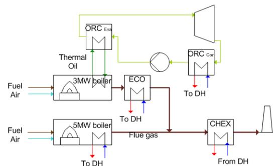
**Figure 1:** Sketch of the plant. DH – district heating, ORC – Organic Rankine Cycle, CHEX – condensing heat exchanger, ECO - economizer
