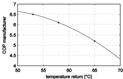
**Figure 5:** Coefficient of performance of the heat pump depending on the inlet temperature of the sink.
