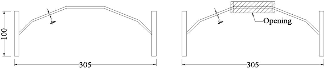
**Fig. 1:** a) Polygonal specimen without opening; b) Polygonal specimen with opening.
