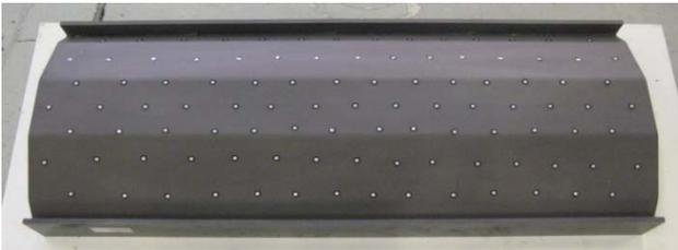
**Fig. 3:** Preparation of specimen surface for scanning geometric imperfections [4].
