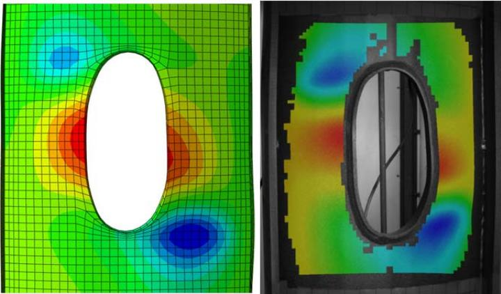
**Fig. 11:** Buckling around opening of the circular specimen with opening (FEA and experimental result).
