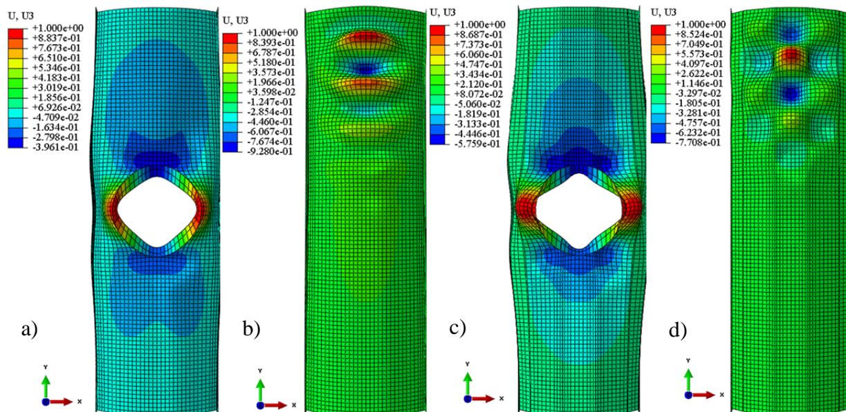
**Fig. 8:** First buckling mode of a) circular model with opening; b) circular model without opening; c) polygonal model with opening and d) polygonal model without opening.
