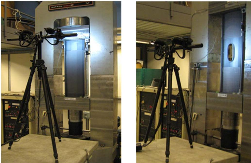
**Fig. 5:** Set-up compression tests with Aramis system.
