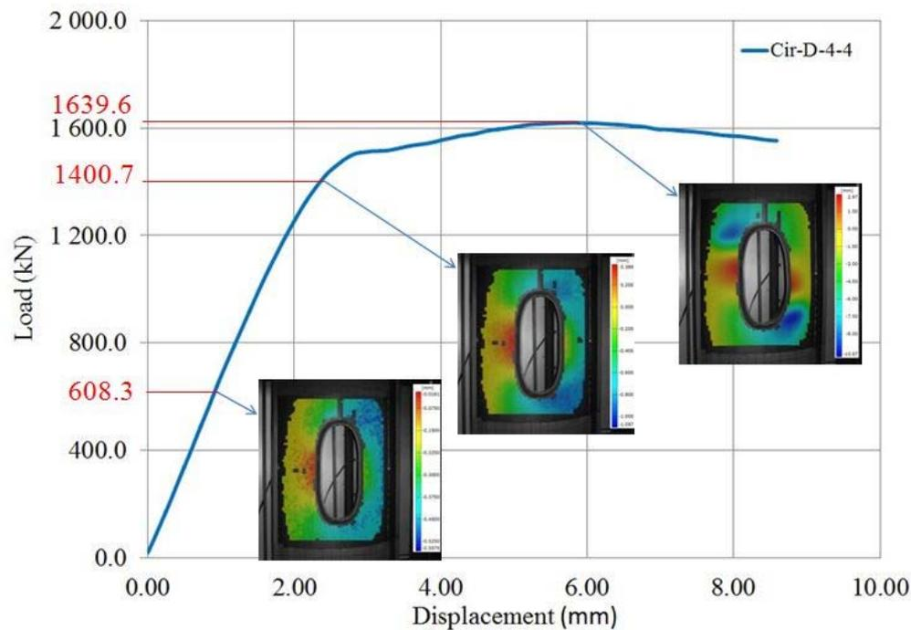
Fig. 12: Buckling development around opening.
