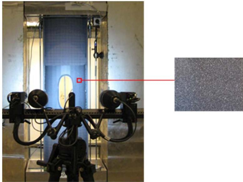
**Fig. 4:** Preparation of specimen surface for buckling observation.
