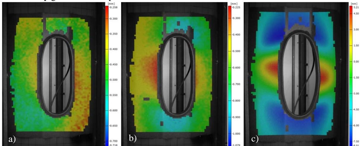
**Fig. 9:** Buckling development around opening of polygonal specimen with opening at applied load: a) 605.8 kN; b) 1400.3 kN; c) 1651.2 kN.
