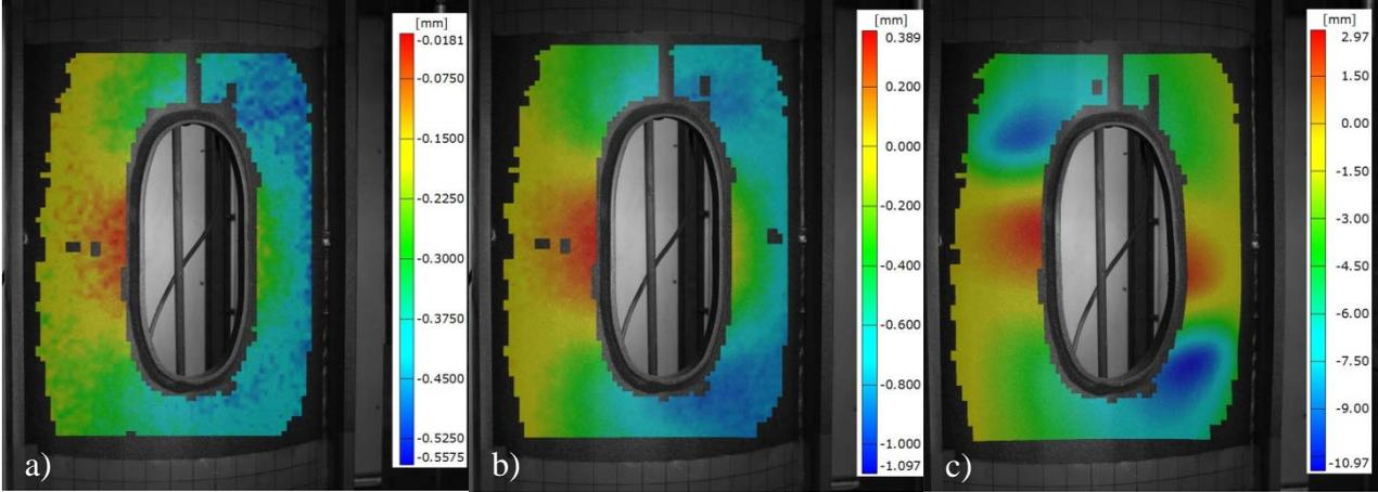
**Fig. 10:** Buckling development around opening of circular specimen with opening at applied load: a) 605.8 kN; b)1400.3 kN; c)1651.2 kN.
