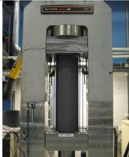
**Fig. 6:** Typical compression test set-up.
