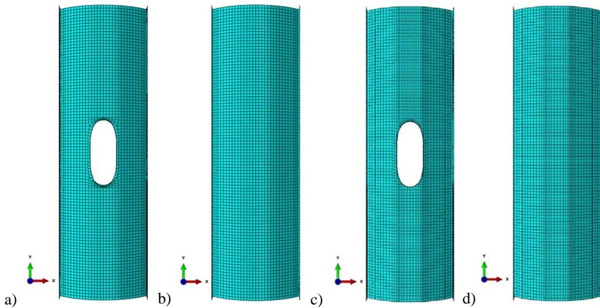
**Fig. 7:** a) circular model with opening; b) circular model without opening; c) polygonal model with opening and d) polygonal model without opening.
