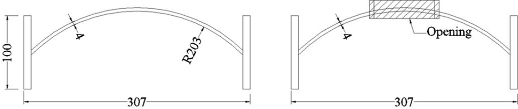
**Fig. 2:** a) Circular specimen without opening; b) Circular specimen with opening.
