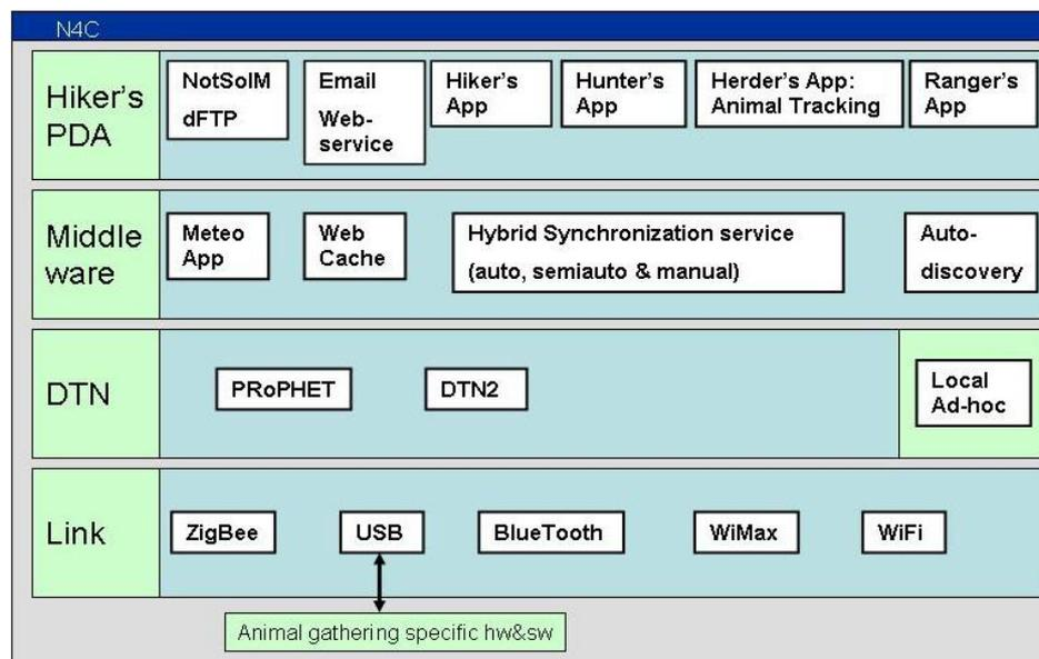
Figure 2. N4C Hiker's Application Software Model with Applications, Middleware, DTN and Link Tiers
