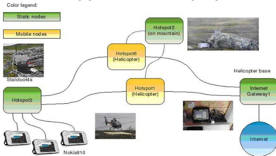
Figure 1: Example topology for summer test in a remote Lappish village using 3 Nokia810. There are 4 hotspots: one in a tent, 2 in helicopters and one on a mountain. The gateway to Internet resides in the helicopter base station in Ritsem.
