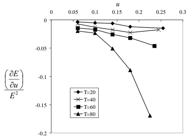
Fig. 1.  $\frac{\left(\frac{\partial E}{\partial u}\right)}{E^2}$  as a Function of Moisture Content  $u$  at Temperatures 20°C, 40°C, 60°C and 80°C (MPa<sup>-1</sup>).
