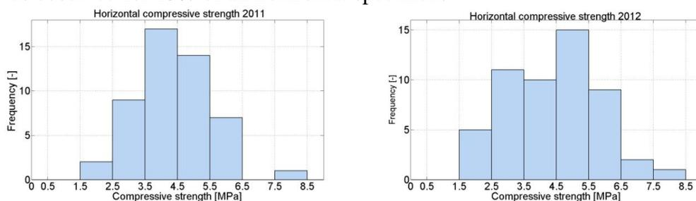
Figure 5. Frequency distributions of horizontal compressive strength.
