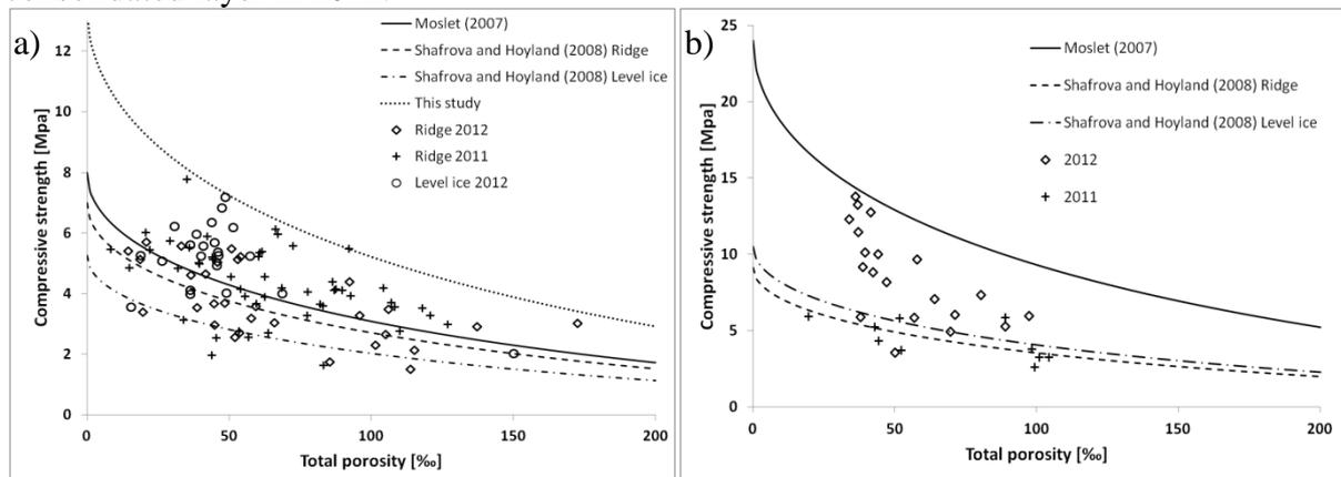
Figure 7. a) Horizontal and b) vertical compressive strength for all tested specimen. The level ice samples are marked with a circle; all other samples are from consolidated layer. Trend lines expressing maximum compressive strength are added from earlier studies.
