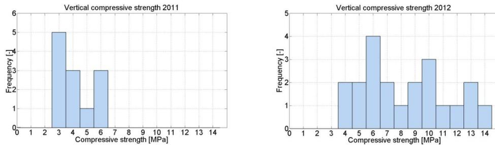
Figure 6. Frequency distributions of vertical compressive strength.
