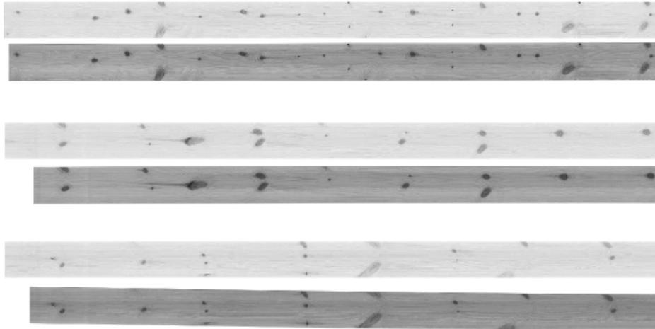
**Figure 1:** Example of a few boards from the floorboard dataset scanned at two different occasions (board lengths have been cropped to fit the page). Dark pixel regions have been cropped away from the rescanned boards (the lower of each image pair) to better show the differences in brightness.
