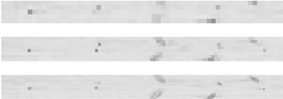
**Figure 4:** Examples of fingerprints of a board downsampled to resolutions 0.04 pixels/mm, 0.08 pixels/mm, and 0.12 pixels/mm (top to bottom). The length has been cropped to fit the page.
