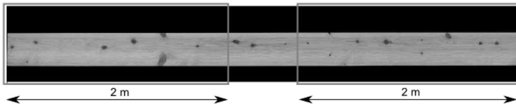
**Figure 3:** The rescanned boards were split into additional images. The pixels inside the rectangles were extracted to become a new dataset. The total board length has been cropped to fit the page.
