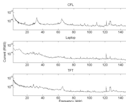
Fig. 4. The spectrum of the current drawn by a CFL upper, Laptop (middle) and TFT screen (lower) between 2 to 150 kHz.
