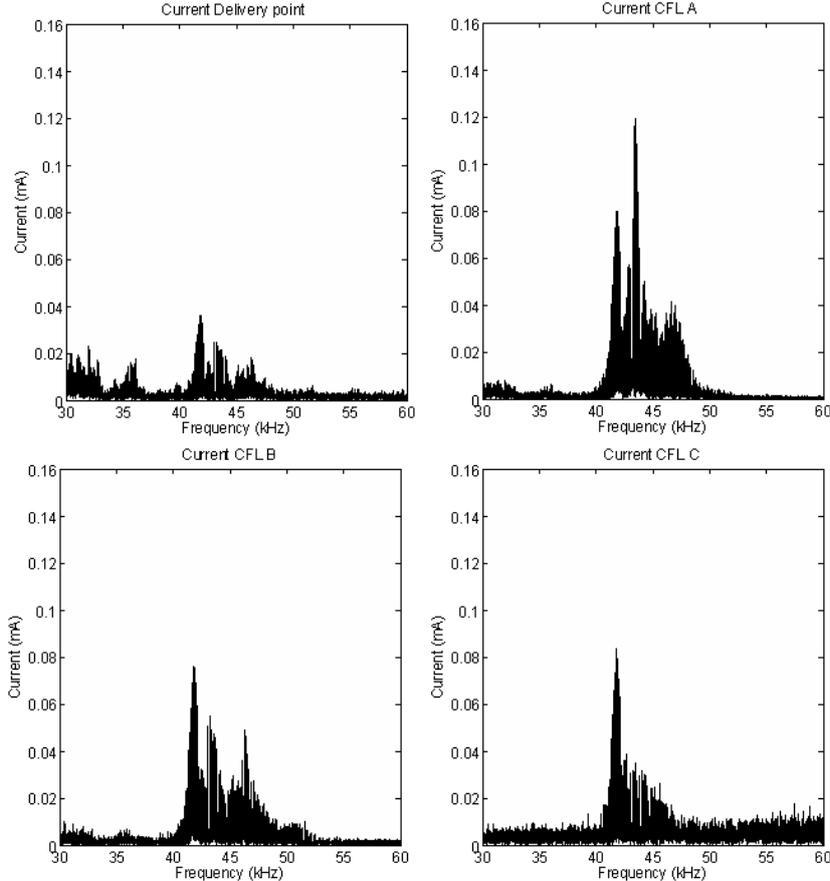
**Figure 5** Supraharmonic current measured at three individual CFLs is shown (upper right, lower left and lower right) and the combined current taken by all three lamps (upper left).
