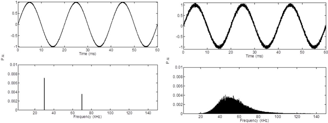
**Figure 1** Example of a narrow band signal in the time domain (upper, left-hand side) and frequency domain (lower, left-hand side) and a broadband signal in the time domain (upper, right-hand side) and frequency domain (lower, right-hand side)
