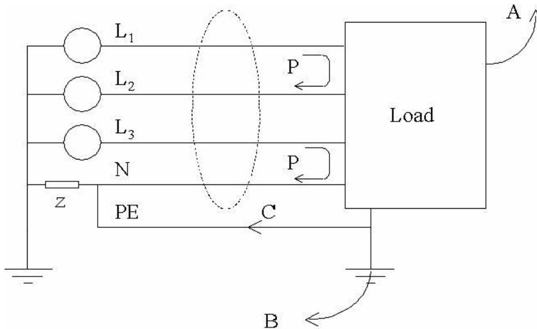
**Figure 3 Different types of emission in a three-phase grid.**
