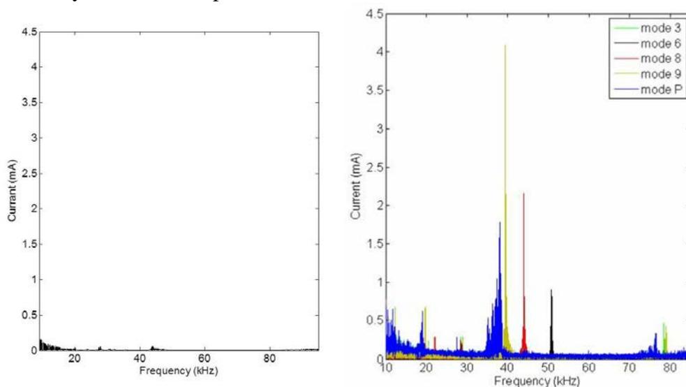
**Figure 4 Primary emission measured at the terminal of a CFL (left hand side). Secondary emission emitted by an induction cooker and absorbed by that same CFL (right hand side).**
