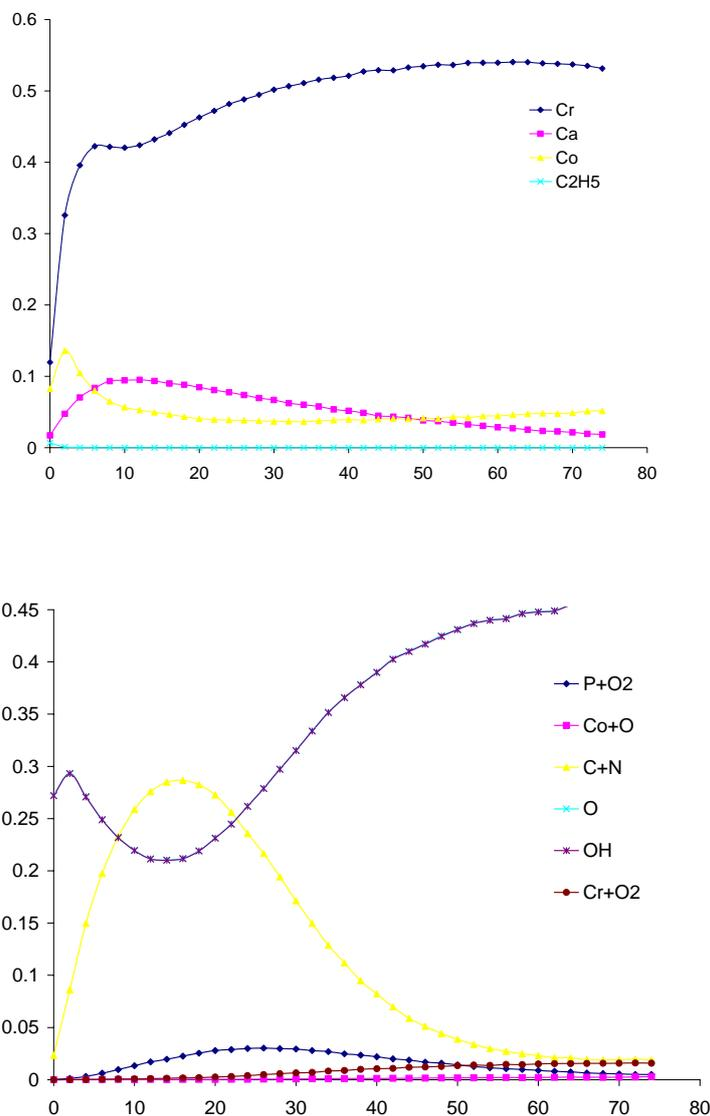
Figures 2 and 3 show the depth profiles (+SIMS and -SIMS) of the Cr, Ca, Co C2H5 and  $PO_2^-$ ,  $CrO_2^-$ ,  $CoO^-$ ,  $O^-$ ,  $CaOH^-$  and  $OH^-$  ions at the surface of the CoCr specimens after immersion in MEM for 10 min and 1h.
