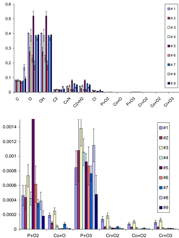
Figure1a and 1b: A typical spectrum (negative SIMS) for CrCo specimens immersed in serum, synovial fluid and MEM for different time intervals.
