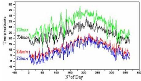
Fig. 5: Daily temperature variation (maximal and minimal) ambient and in the ground for Tlemcen site
