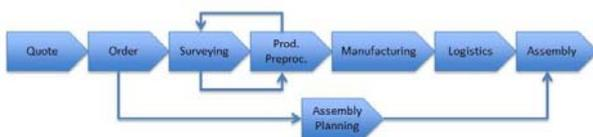
**Figure 1:** The value stream from quote to assembly.
