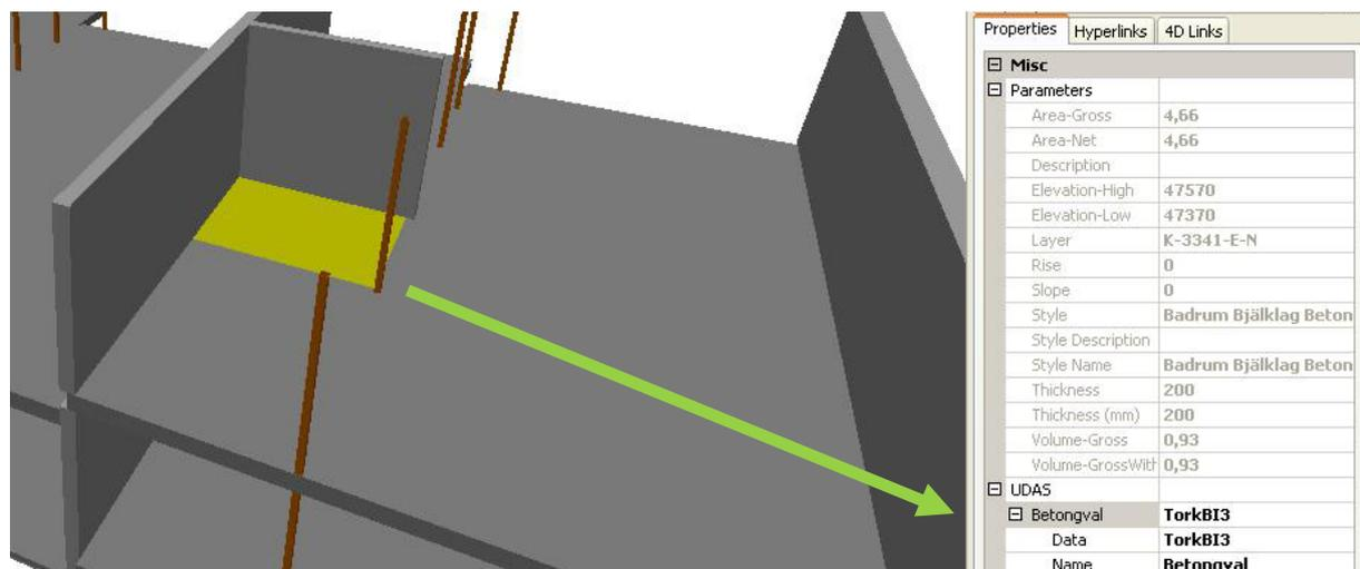
FIG. 3: A selected object containing data about the concrete quality and its volume.
