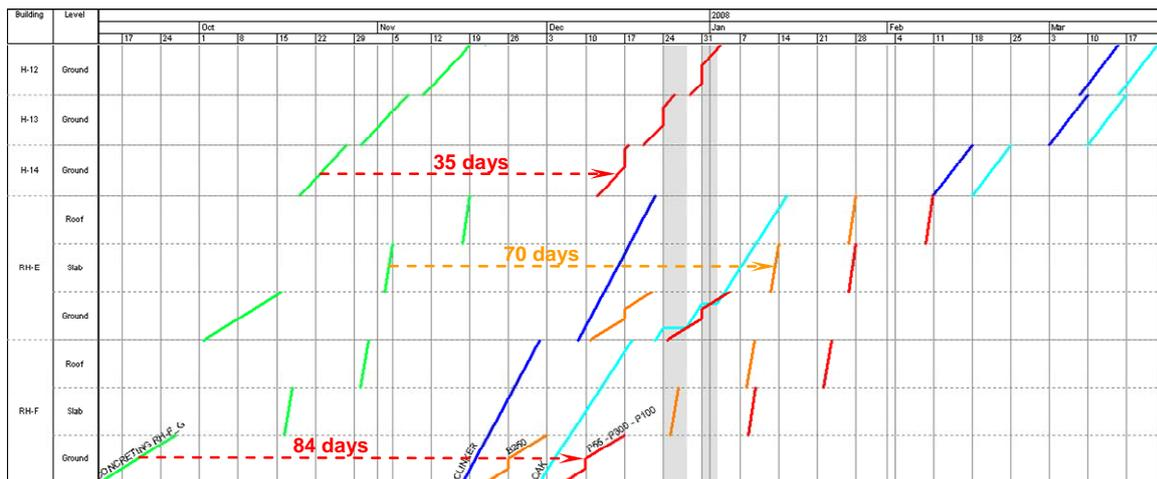
FIG. 2: Location based desiccation simulation for phase 1.
