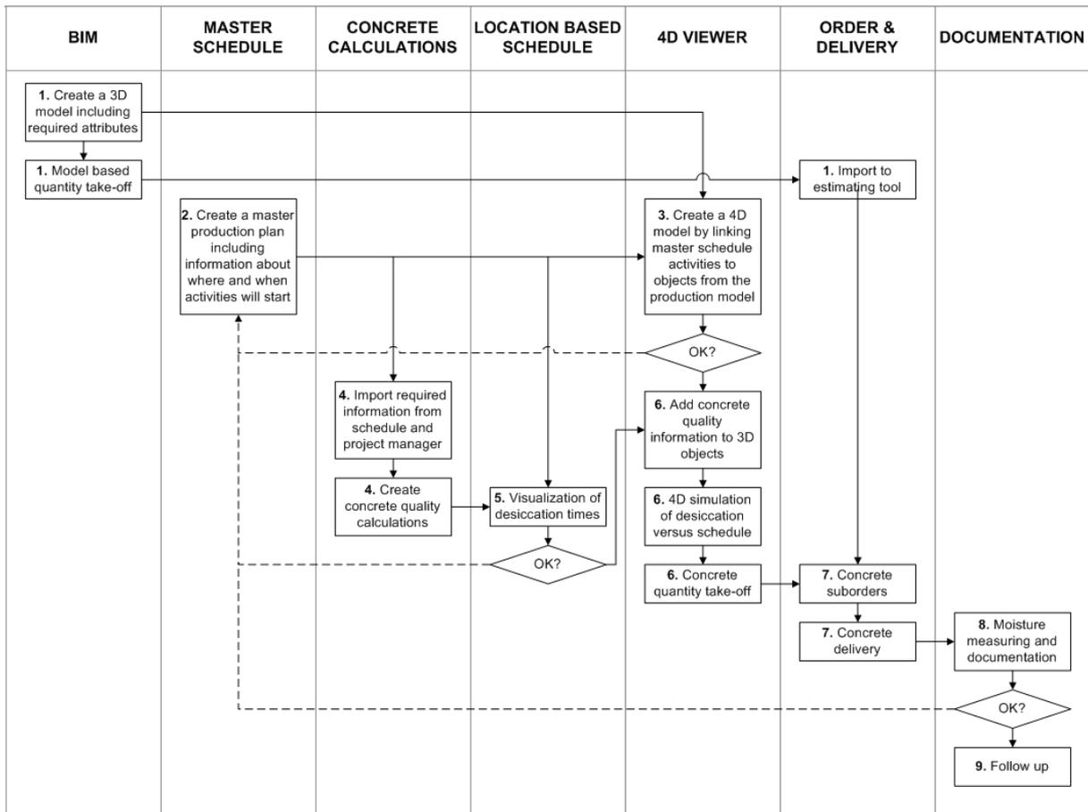
FIG. 4: A proposed process method to support cast in place concrete construction using model- and location-based techniques.
