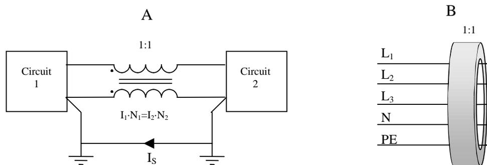
**Figure 6.** Common- mode choke acts like a 1:1 current transformer balancing the current to be alike. The current that flows in one wire prefers to go back in the other wire instead of using any other ( $I_s$ ) way. One common way to make that 1:1 transformer is to use a toroid core (B) and put the signal line or power line through the hole.
