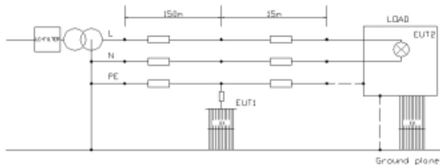
Figure 7. Set-up for measurements on light fittings
