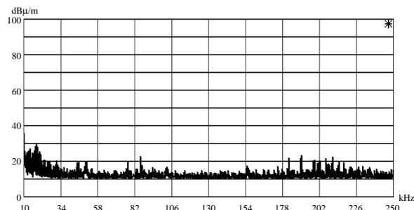
**Figure 9.** Showing the background noise when six light bulbs are connected as a load.
