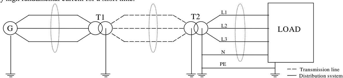
**Figure 1.** The transport of energy in a three-phase distribution system. The neutral line N is only used for one-phase load. The protected earth system including PE-wire meet security aspects for both human beings and properties. The sum of the currents enclosed by the dotted circle shall under normal operating conditions be zero.
