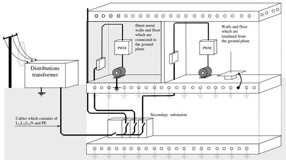
**Figure 5.** Grounding system for a building. The distribution transformer has a grounding point for the grid. Also, the fundament for the building acts like a grounding point at the same time as it functions as a ground plane for the entire installations. Depending on how the electrical equipment is connected to the ground plane, different situations arise in the electrical field. Measurements according to MIL-STD 461D are made with respects to the floor ground plane in the room.
