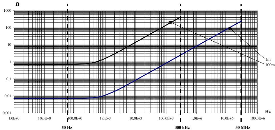
**Figure 4.** Showing the impedance for 2.5 mm<sup>2</sup> Cu -wire with a length of 1 m and 100 m.
