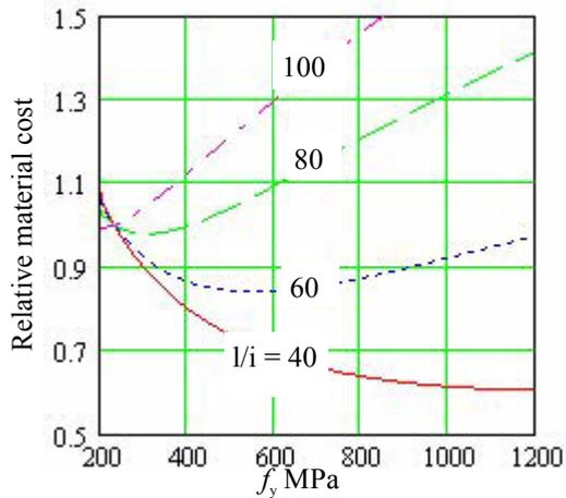
Fig. 3. Relative material cost for column subject to flexural buckling (curve a) as function of yield strength  $f_y$ . Reference cost is for steel S235.
