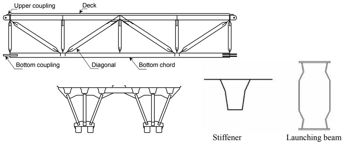
Fig. 11. Truss element for Fast Bridge 48 developed by Karlskronavarvet AB, Sweden.
