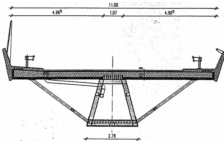
Fig. 8. Cross section of the Nesenbachtalbrücke.
