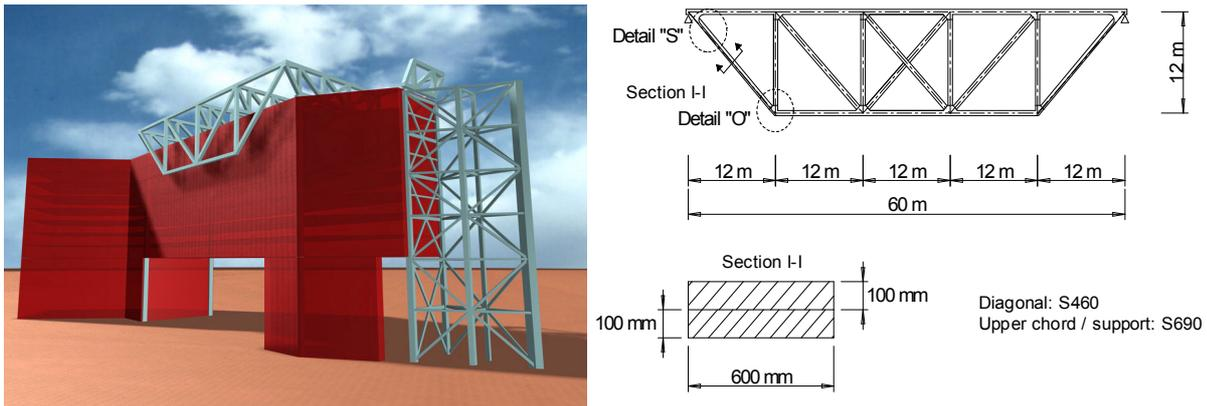
Fig. 9. Truss structure in the Sony Center.
