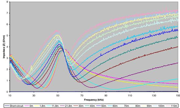
Figure 9, Shunt impedance of the computer with different cable lengths
