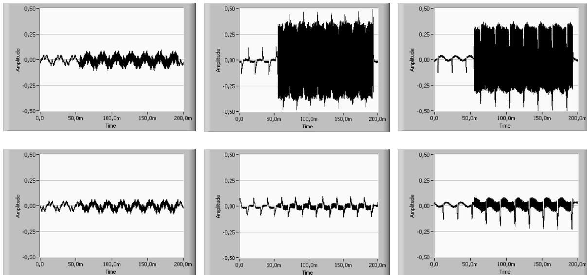
*Figure 11, Currents during power line communication using PLT-30. Upper row of figures is the lamp with an earlier manufacturing date. From left to right, Concentrator, 4W energy saving lamp and Power Meter Transceiver.*
