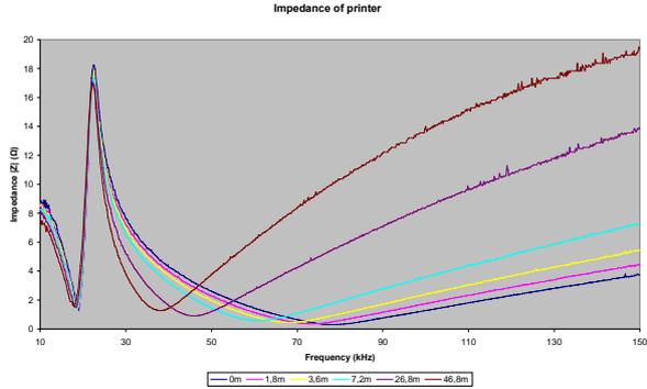
Figure 8, Shunt impedance of the printer with different cable lengths
