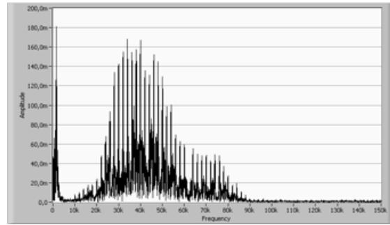
*Figure 5, The non-attenuated signal from Enermet's wideband communication system, PLT-30*
