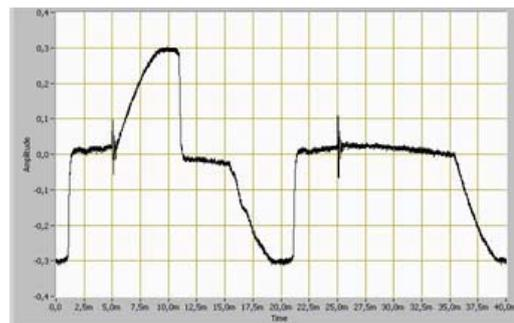
*Figure 12, High frequency, high amplitude oscillation causing the missing half-cycle*
