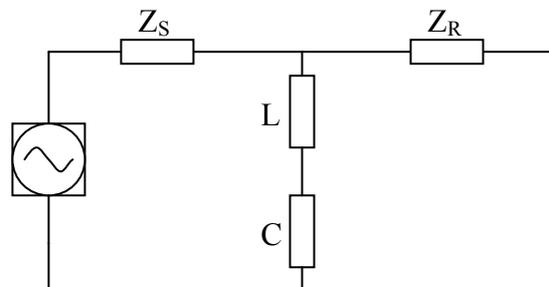
*Figure 7, Measuring the filter effect of equipment*
