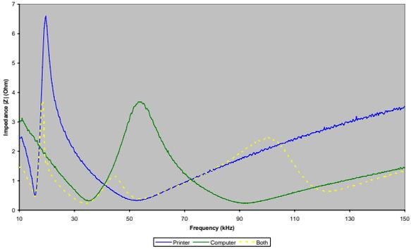
Figure 10, Shunt impedance of printer, computer connected simultaneously
