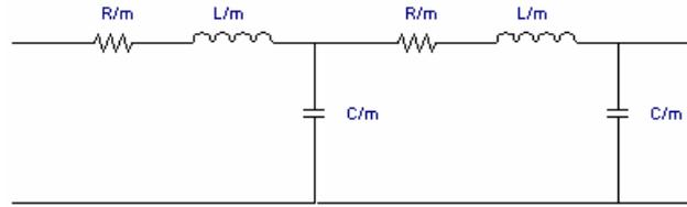
Figure 1, The power line as a distributed RLC network
