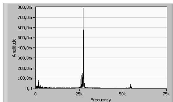
*Figure 3, A possible interfering signal originating from an UPS, amplitude in volts*
