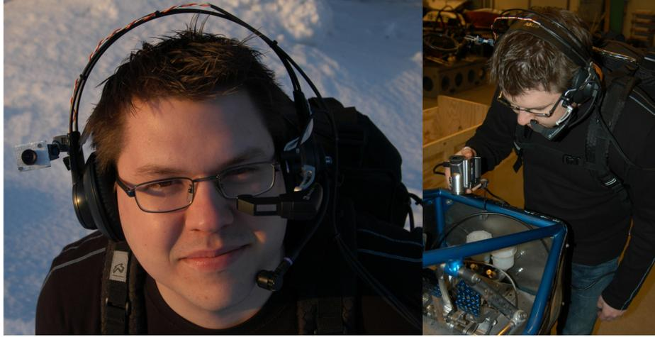
**Fig. 3.** The Boblbee Computer, left picture: close up on the head worn equipment. Right picture: The wearable computer in use at a mock-up
