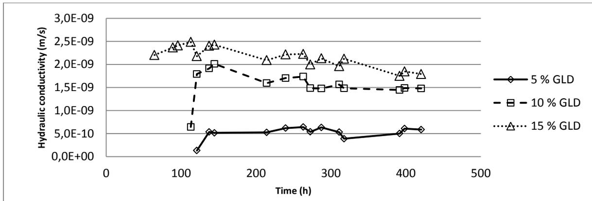
Figure 2. Hydraulic conductivity (HC) in till with 5, 10 and 15 wt. % of added GLD. The HC increases with increasing percentage of GLD added to the till.
