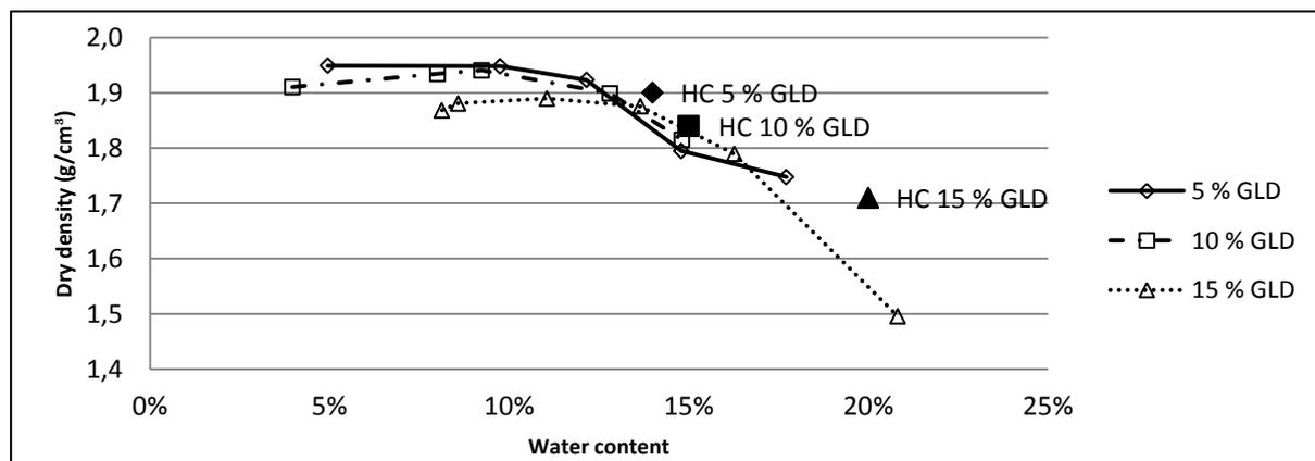
Figure 1. Dry density with increasing water content after proctor compaction in sieved fine grained till with 5, 10 and 15 wt. % of added GLD. The optimal density decreases with an increasing percentage of GLD added to the till. The filled dots marked with HC represent the samples which were proctor- (5 and 10 % GLD) and hand compacted (15 % GLD) for hydraulic conductivity.
