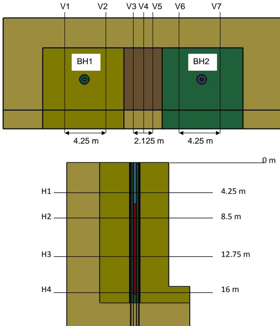
Figure 4. Vertical (top) and horizontal (bottom) evaluation cuts used for results presentation.
