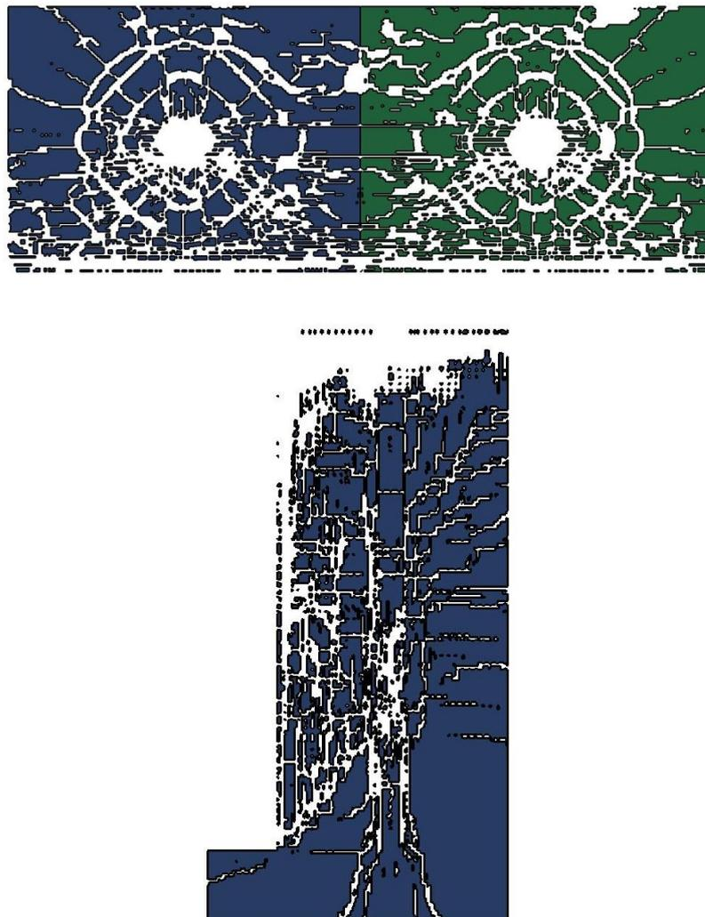
Figure 6. Fragmentation pattern for horizontal cut H1 (top) and vertical cut V4 (bottom); see Figure 4 for location of evaluation cuts. White areas are considered to be fully crushed (damage level > 60 % and thus a fragment size less than 50 x 50 mm).
