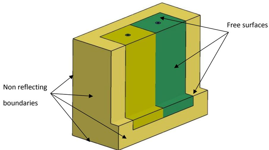
Figure 2. Boundary conditions for the finite element model using LS-DYNA.
