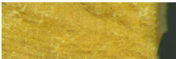
**Figure 2.** Bond surface with paper fibres after failure
