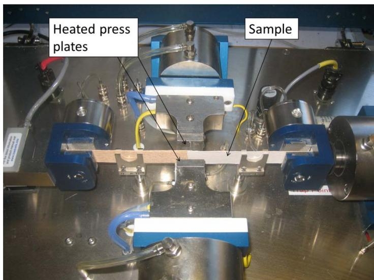
**Figure 1.** Automated bonding evaluation system testing machine
