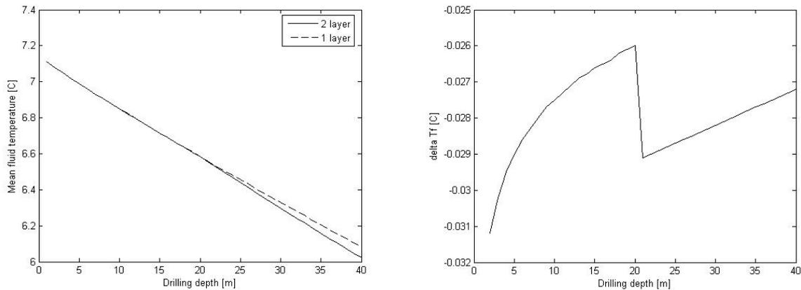
Figure 4: a) mean fluid temperature for two different bedrocks, layered ( $\lambda_1 = 3$  W/m,K and  $\lambda_2 = 4$  W/m,K) and non-layered ( $\lambda = 3$  W/m,K) b) drilling depth derivative of mean fluid temperature for the layered bedrock.
