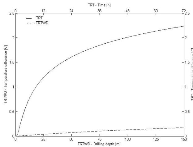
Figure 3: Temperature difference between simulations with conductivity 3 W/m,K and 4 W/m,K,  $T_f(\lambda = 3) - T_f(\lambda = 4)$ , for the TRT and TRWD.
