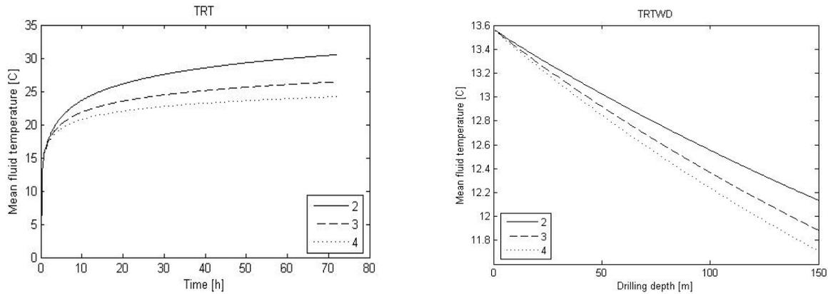
Figure 2: Simulation results for a) TRT measurement and b) TRTWD measurement for three different bedrock conductivities;  $\lambda_1 = 2$  W/m,K,  $\lambda_2 = 3$  W/m,K and  $\lambda_3 = 4$  W/m,K.
