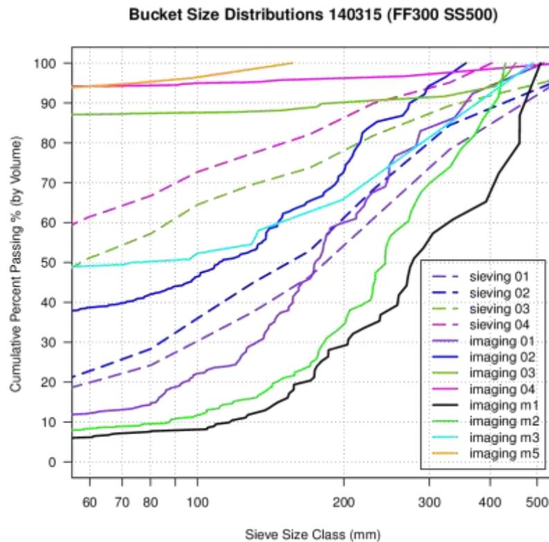
Figure 18. Cumulative size distribution curves for LHD buckets, 4 sieving, and 8 imaging curves.
