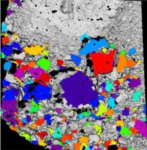
Figure 10. 3D draw-point 03, non-overlapped rocks in colour
