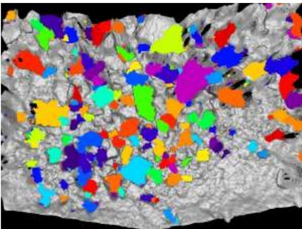
Figure 14. 3D bucket 02, non-overlapped rocks colour
