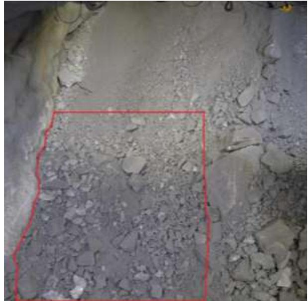
Figure 9. Draw-point 04 with LHD bucket 04 excavated area
