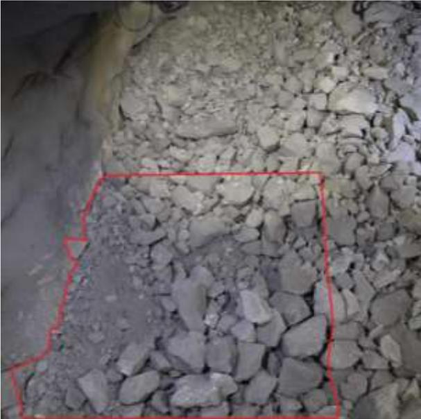
Figure 6. Draw-point 01 with LHD bucket 01 excavated area
