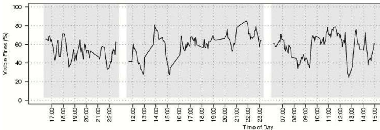
Figure 19. Percentage of the surface identified as areas-of-fines for 424 LHD production bucket loads (Thurley, 2009)
