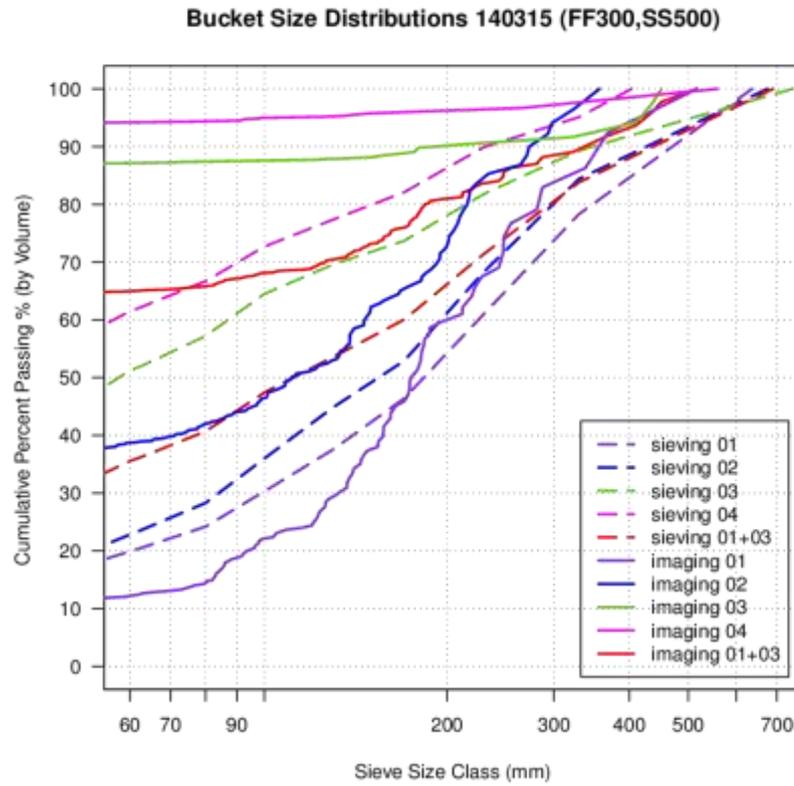
Figure 17. Cumulative size distribution curves for LHD buckets 01,02,03,04
