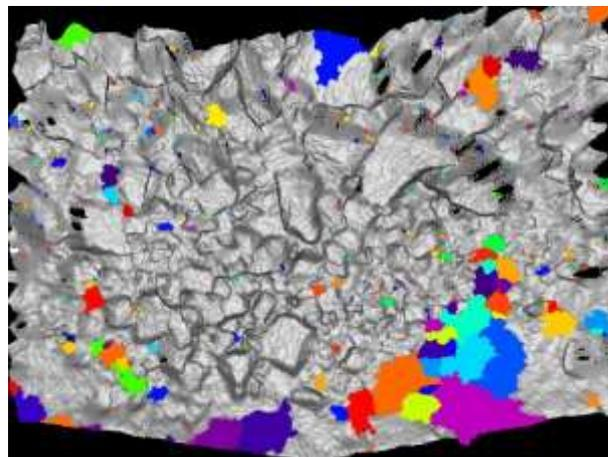
Figure 15. 3D bucket 02, areas-of-fines in colour
