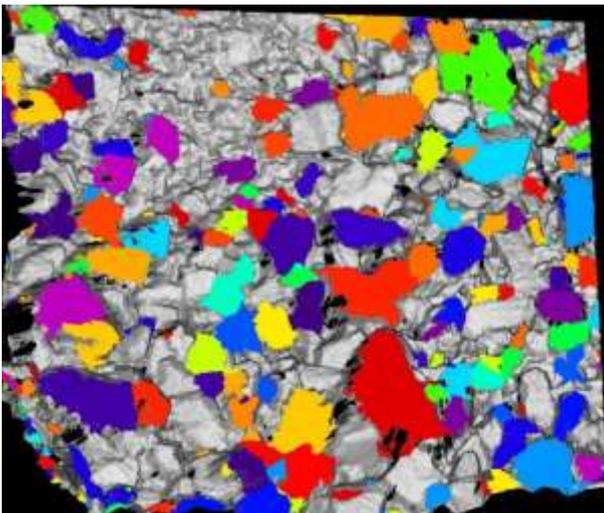
Figure 12. 3D draw-point 02, non-overlapped rocks in colour
