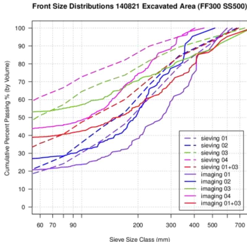
Figure 16. Cumulative size distribution curves for draw-points 01,02,03,04
