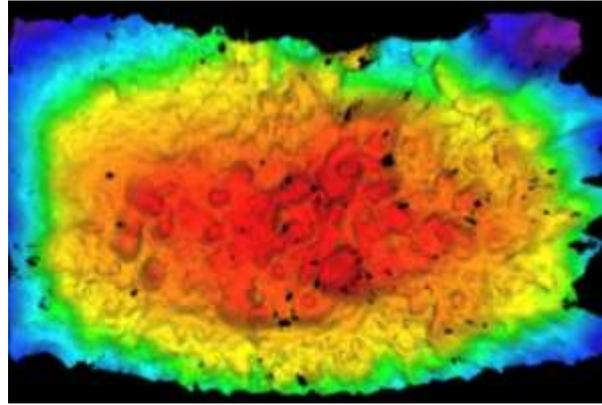
Figure 21. LHD bucket 3D data set m5, with colouring based on the height (red highest, blue & purple lowest)
