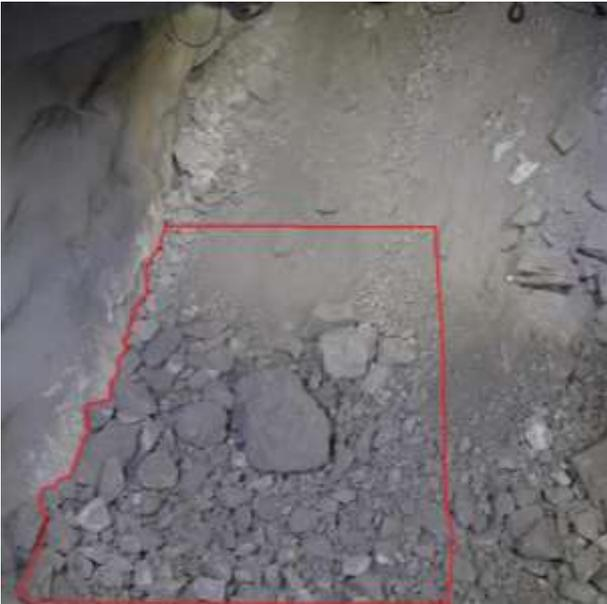
Figure 8. Draw-point 03 with LHD bucket 03 excavated area
