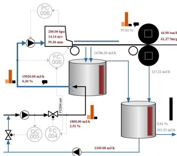
**Figure 4 Graphical interface of stock preparation process to press section.**
