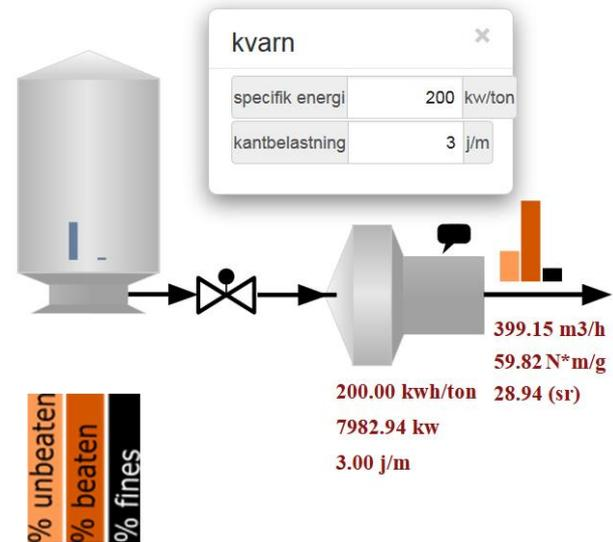
**Figure 3 Refiner interface (kvarn in Swedish) with input dialog box open.**
