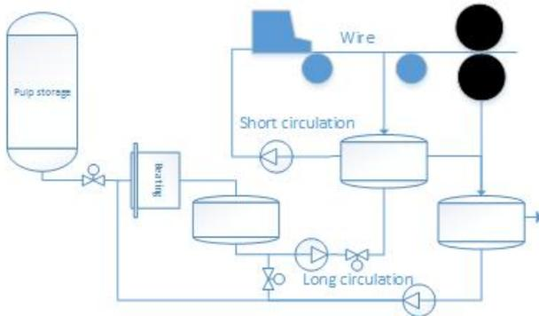
Figure 1, Stock preparation process to press section.
