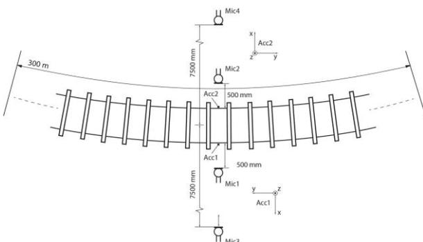
**Figure 13: The measurement setups illustrating the mounting for Mic. 1-4 and Acc. 1 & 2 [25].**
