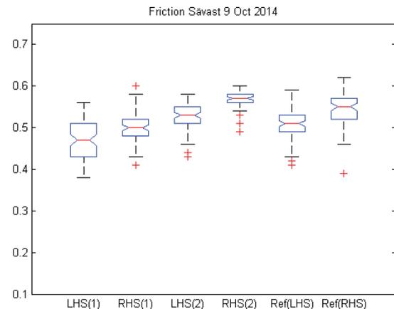
**Figure 10: Friction coefficient measured at facility 2 on 9 Oct 2014.**
