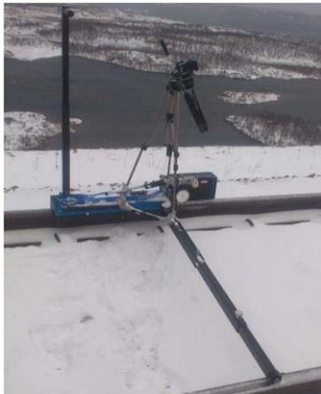
**Figure 8: The manually pushed tribometer used to determine the friction.**
