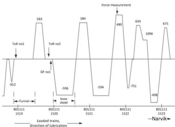
**Figure 6: The track geometry of test facility 1, loaded trains running in the direction towards Narvik.**
