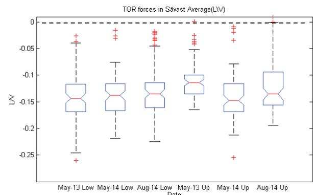
Figure 12: The average L/V for facility 2, before the start of the TOR lubrication, after one year, and after one year and three months.
