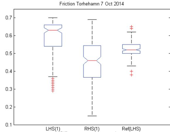
**Figure 9: Friction coefficient measured at facility 1 on 7 Oct. 2014.**
