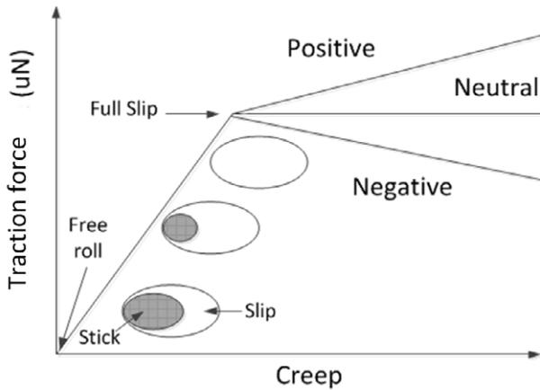
**Figure 4: Different types of friction behaviour, adapted from [19, 20].**
