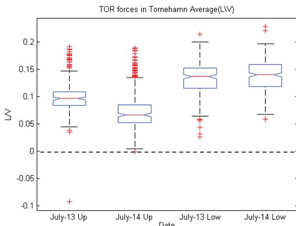
Figure 11: The average L/V for facility 1, before the start of TOR lubrication and after one year of service.
