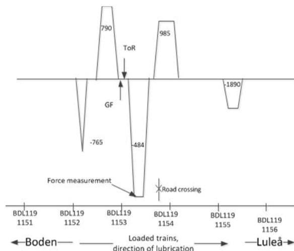
**Figure 7: The track geometry of facility 2, loaded trains running in the direction towards Luleå.**
