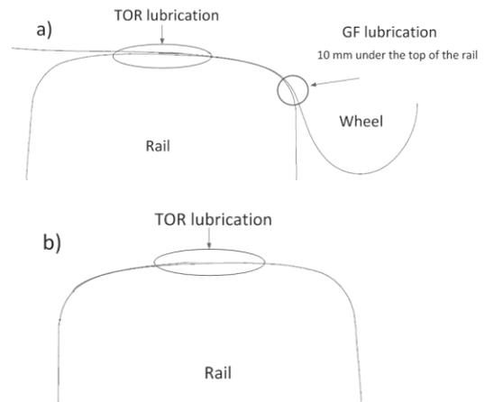
**Figure 3: a) Application of TOR and GF lubricant on the upper rail in curves.
