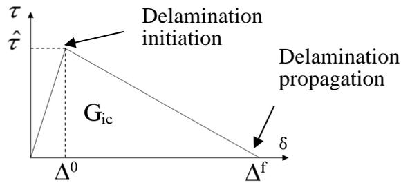
Figure 1. Bilinear traction separation law.
