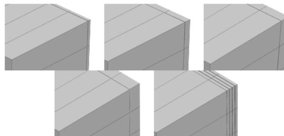
Figure 4. The five models with cohesive elements positioned at different composite layer interfaces on the tension side
