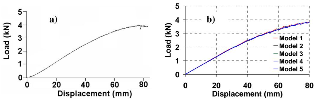
Figure 5. Load-displacement curves – a) Experiment [5]; b) FE models
