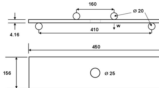
Figure 2. Geometry of the notched composite plate (mm)
