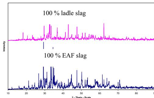
**Figure 1.** Diffraction pattern of 100 % ladle slag and 100 % EAF slag
