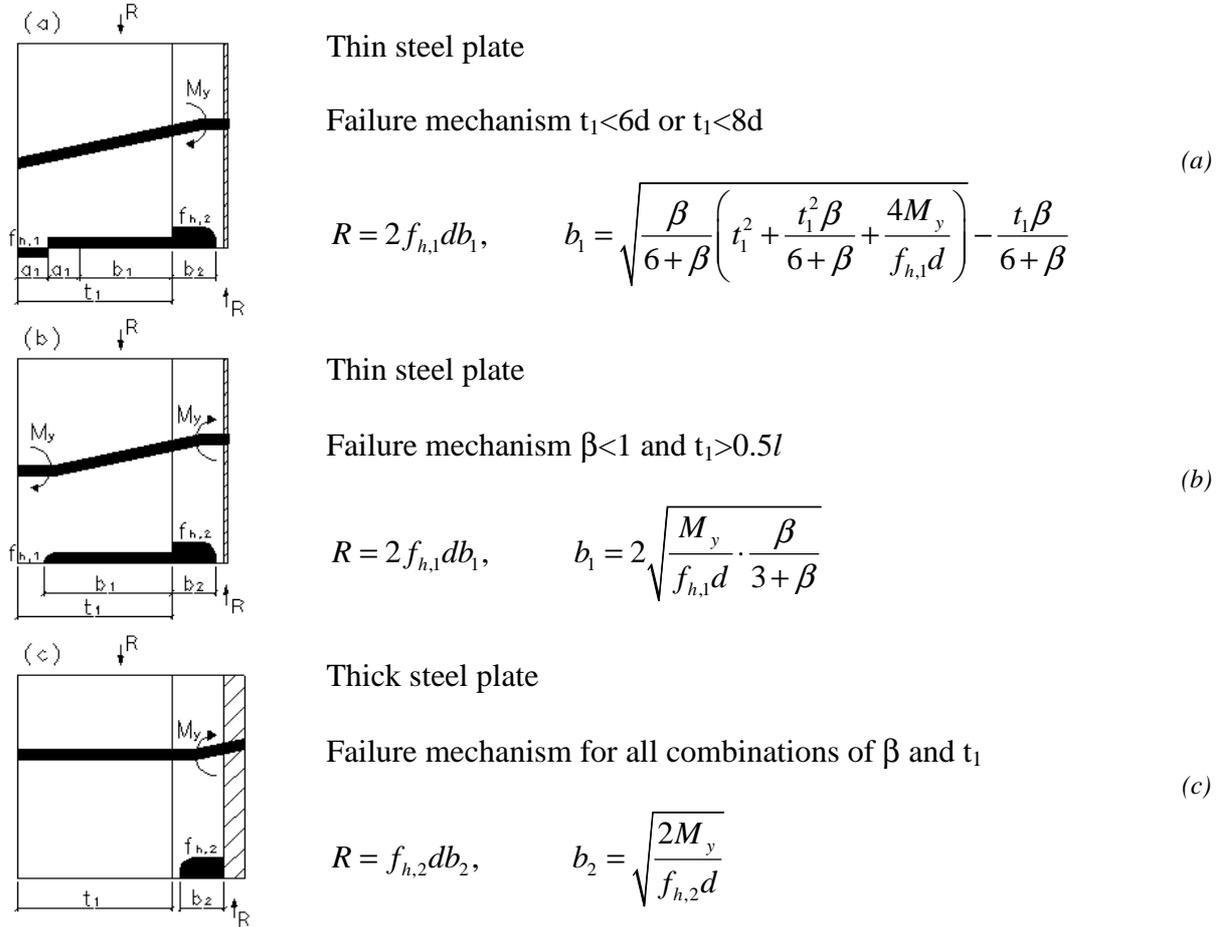
Figure 1 Assumed failure mechanisms: (a, b) Thin steel plate with thick interlayer, (c) Thick steel plate with thick interlayer
