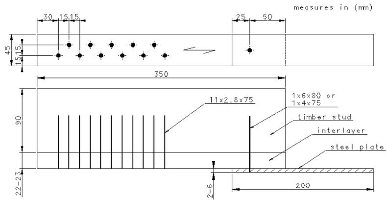
Figure 2 Test set-up of the single shear timber-interlayer-steel plate joints
