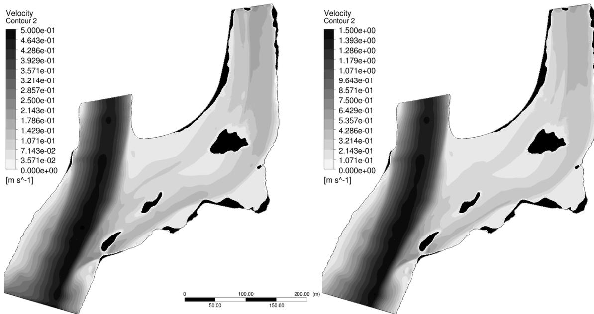
Figure 3. Velocity contours at 1 m depth for 200 m<sup>3</sup>/s, 20 m<sup>3</sup>/s spill (left) and 600 m<sup>3</sup>/s, 50 m<sup>3</sup>/s spill (right). Areas with depth < 1 m are marked with black color.
