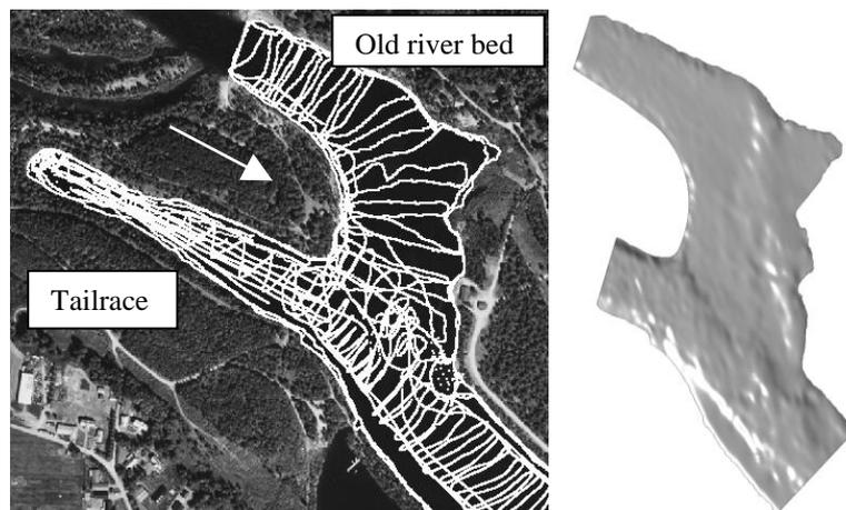
Figure 1. Measured depth data for geometry creation and the simulation domain
