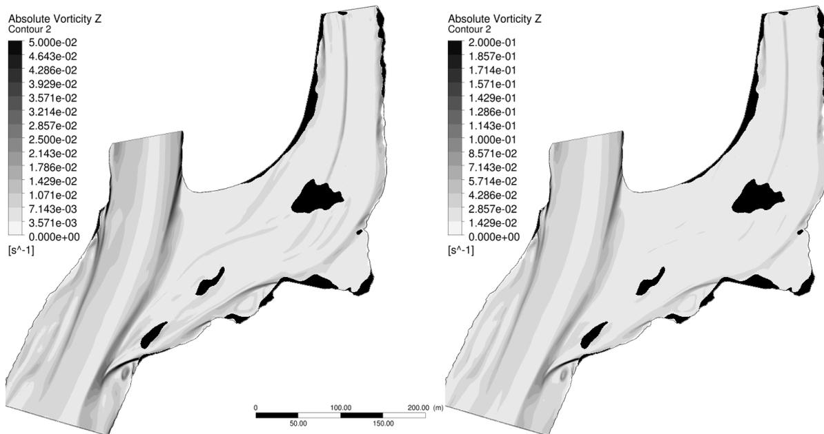
Figure 4. Absolute vorticity at 1 m depth for 200 m<sup>3</sup>/s, 20 m<sup>3</sup>/s spill (left) and 600 m<sup>3</sup>/s, 50 m<sup>3</sup>/s spill (right). Areas with depth < 1 m are marked with black color.
