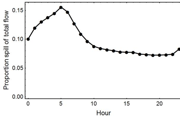
Figure 7. The average daily pattern of spill in relation to total flow displayed a peak around 5 am and remained low from 10 am to 10 pm.
