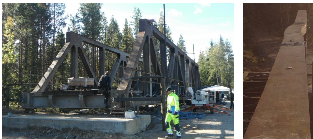
Figure 3. Test of a metallic bridge. Overview of test site with two jacks anchored in the bed rock in the centre (left) and final buckling failure of top girder beam (right), Häggström and Blanksvärd [6].
