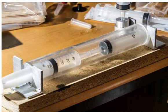
Figure 1. Grease mixing jig.
