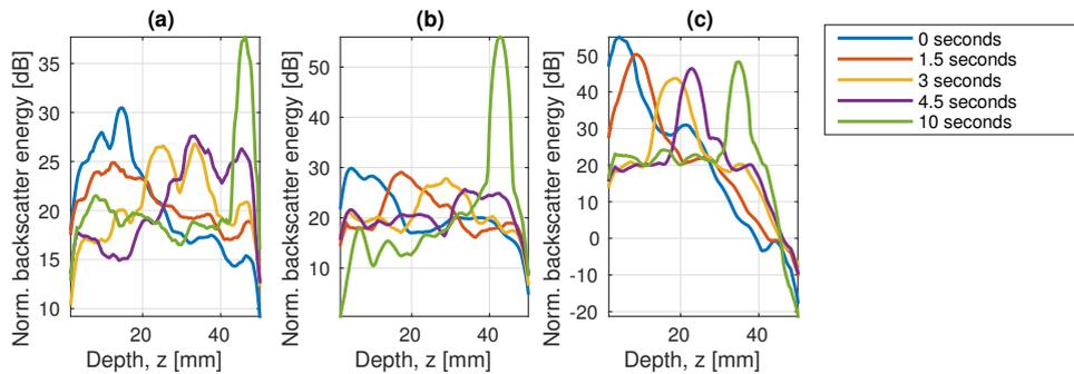
Fig. 4. Slices from Fig. 3, taken 0 s, 1.5 s, 3 s, 4.5 s, and 10 s after the settling process started, for solids concentrations of (a) 1.7 vol%, (b) 4.0 vol%, and (c) 6.7 vol%
