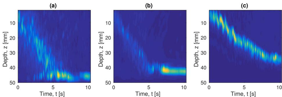
Fig. 3. Energy of backscattered ultrasound as function of the settling time,  $t$  for solids concentrations of (a) 1.7 vol%, (b) 4.0 vol%, and (c) 6.7 vol%.
