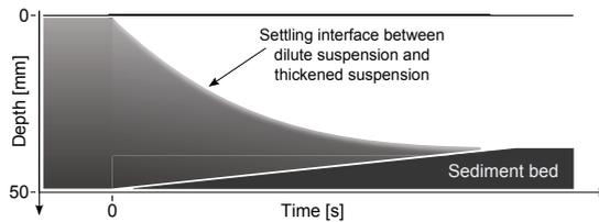
Fig. 1. Sketch of suspension settling, dark color indicates high particle concentration. Before time 0 a turbulent flow of suspension goes through the flow cell. As the pump is decelerated to a stop the suspension starts to settle, and a sediment bed begins to form on the bottom of the cell.
