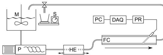
Fig. 2. Experimental setup consisting of mixer (M), pump (P), heat exchanger (HE), flow cell (FC). Also sampling position (S) and data acquisition equipment; pulser-receiver (PR), digitizer (DAQ) and computer (PC), is shown.
