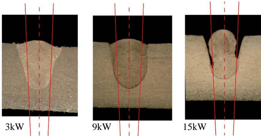
**Fig 10.** Cross-cuts at different welding speed / laser power.
