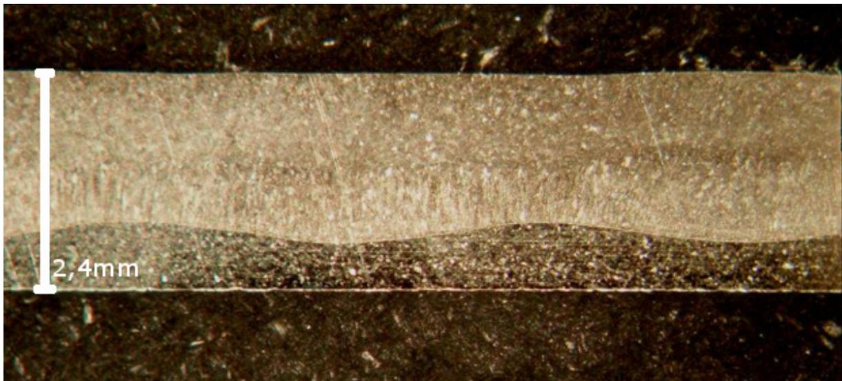
**Fig 9.** Etched cut along weld. 9kW laser power, 9m/min welding speed (150mm/s)
