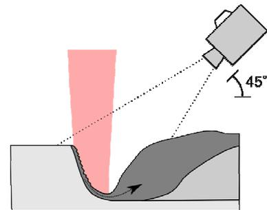
**Fig 2.** Schematic setup, side view of keyhole and melt pool
