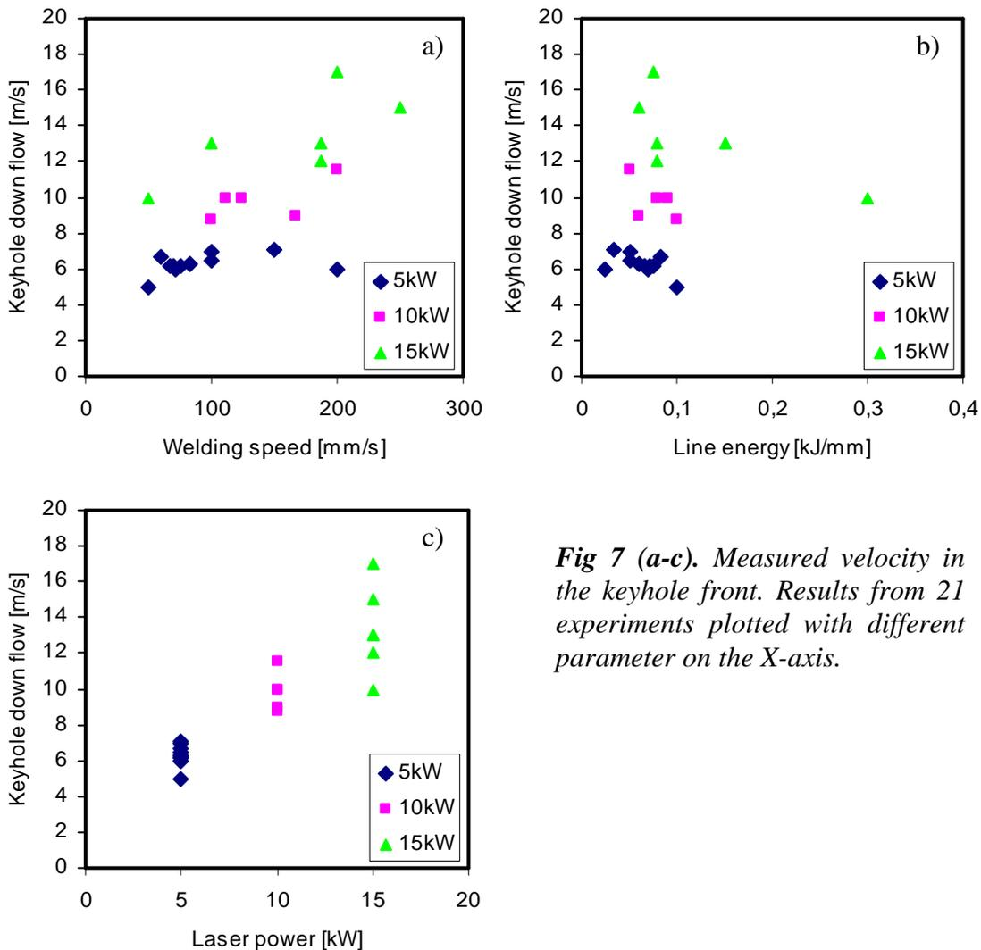
**Fig 7 (a-c).** Measured velocity in the keyhole front. Results from 21 experiments plotted with different parameter on the X-axis.
