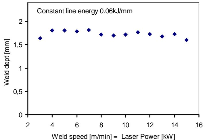
**Fig 8.** Weld depth measured from cross-cuts.
