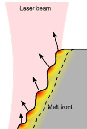
*Fig 12. Locally heated bumps with evaporation pressure normal to the surface*
