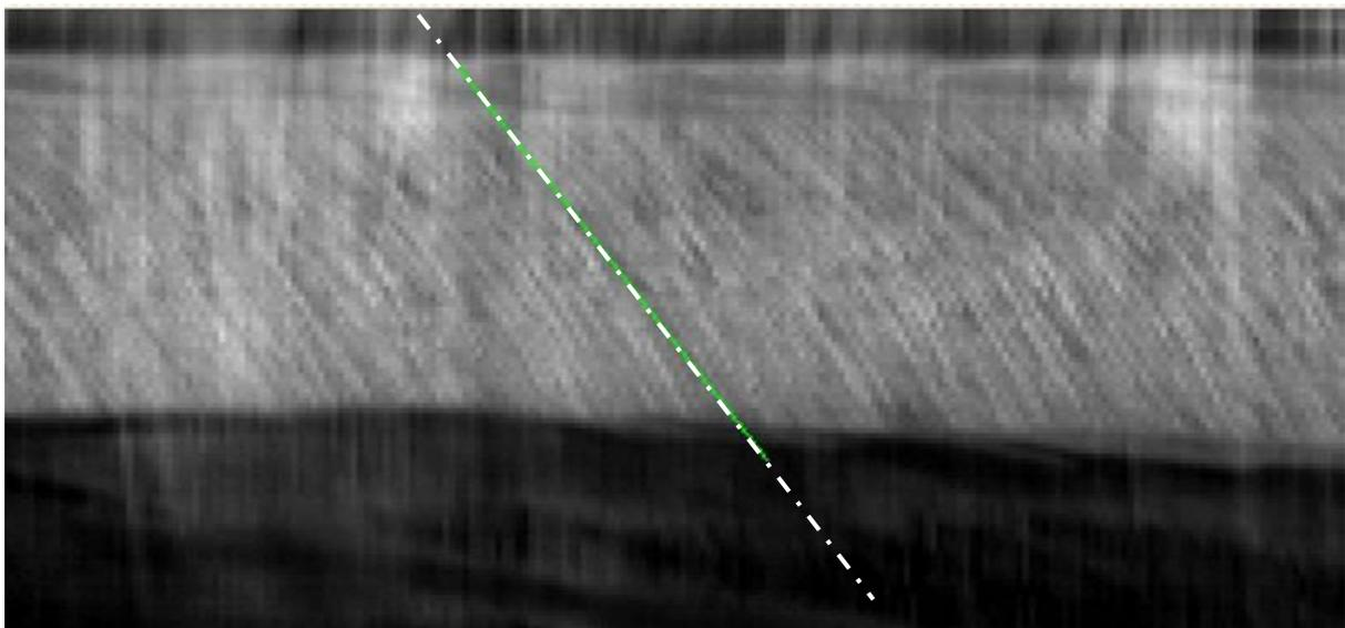
**Fig 5.** Streak image from 255 frames Dashed line represents 8,4m/s velocity
