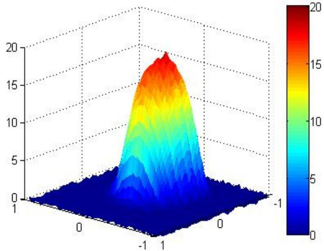
**Fig 1.** Beam profile on top surface at 800W laser power with -9mm focus position
