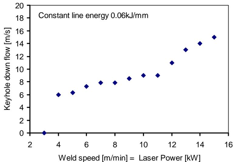
**Fig 11.** Downward flow during welds with line energy of 0.06kJ/mm
