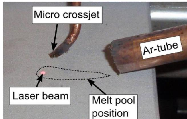
**Fig 3.** Position of micro crossjet
