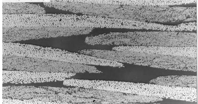
Fig.1. Cross-section of a moulded fibre reinforced composite material. The white and light grey areas are fibres in different directions while the dark grey area denotes the solidified resin. The diameter of the fibres is about 5  $\mu\text{m}$ .
