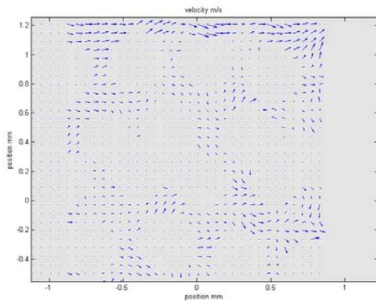
Fig.14. Velocity field near bottom of the channel.
