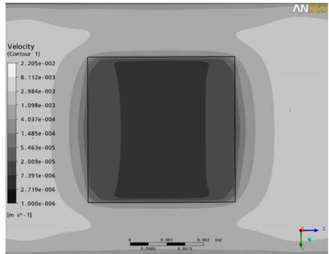
Fig.3. Contour plot of the velocity in the flow direction for fibre bundle and surrounding flow in the symmetry plane.
