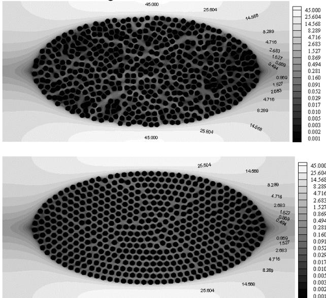
Fig.5. Contours of flow speed in two systems having different intra-tow fibre distributions. (top)  $\delta_1/R=0.05$ , (bottom)  $\delta_1/R=0.295$ . The geometrical parameters of the two systems are otherwise the same ( $\phi_f=0.5$ ,  $\phi_t=0.7$ ,  $N_f=500$  and  $\lambda=2$ ).
