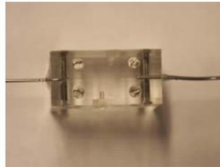
Fig.7. Flow cell, showing the inlet/outlet pipes.
