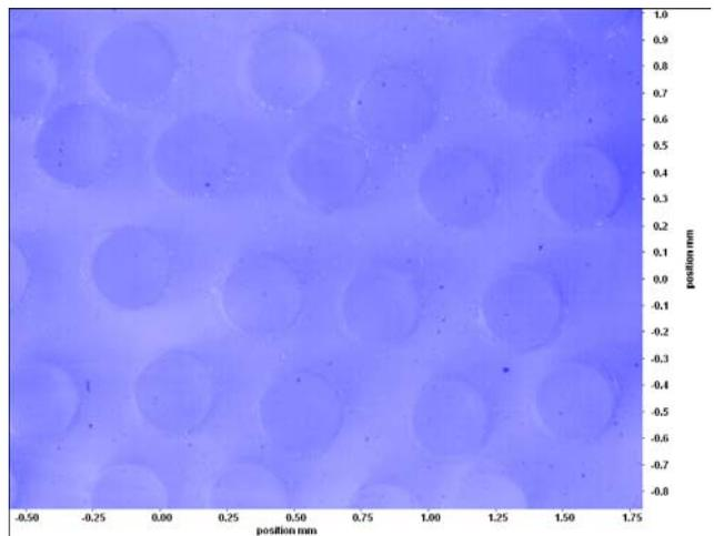
Fig.8. Image of a section of the fibre array obtained using 10x magnification. The bulk flow is in the direction perpendicular to the fibre axes.
