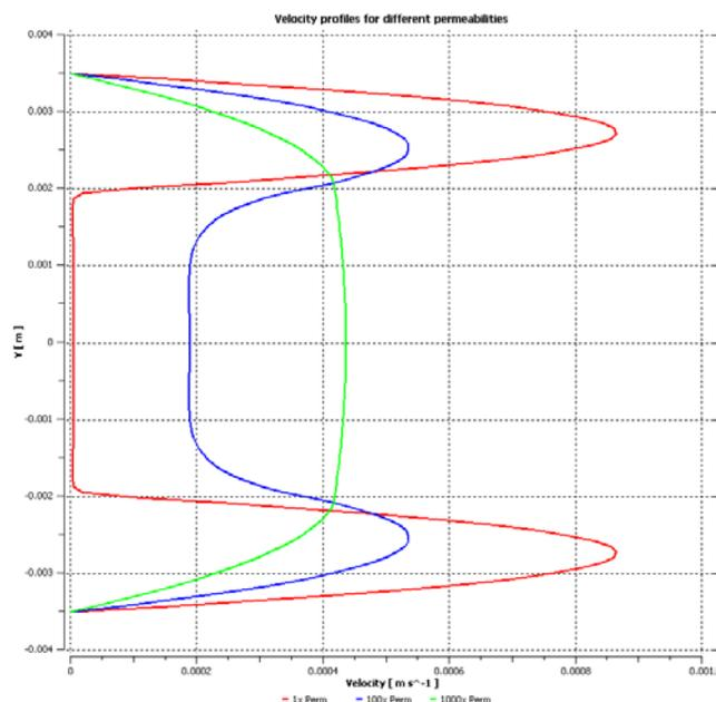
Fig.4. Velocity profiles for different permeabilities in the center of the bundle in the symmetry plane.
