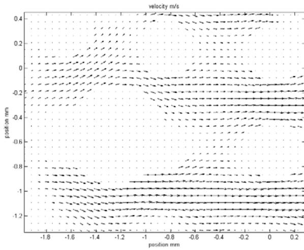
Fig.13 Velocity field for flow around air bubble in a rectangular fibre array
