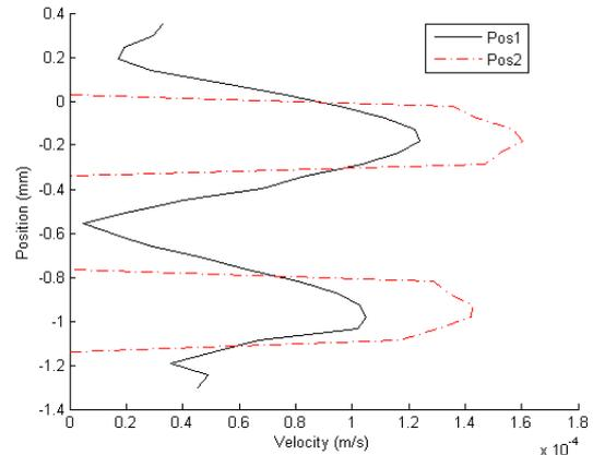
Fig.11 Velocity profiles for min and max cross-section area
