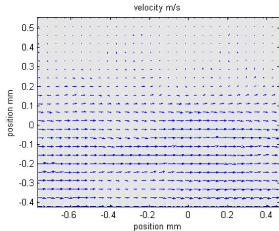
Fig.16. Velocity field near the middle the channel at the border of the array.
