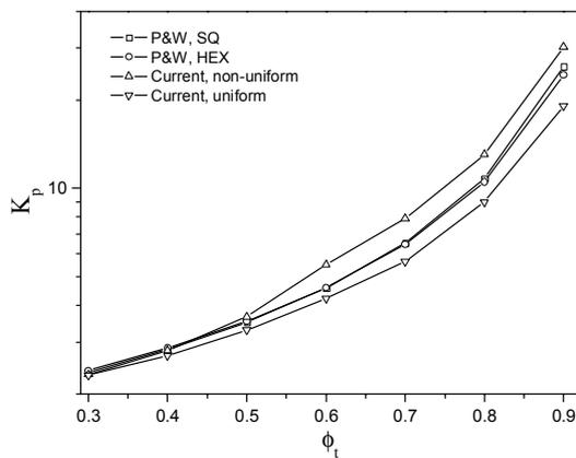
Fig.6. Comparison of the predictions of the Phelan-Wise model (P&W) with numerical results for  $\phi_f=0.40$ . The other conditions are  $\lambda=1$ ,  $N_f=500$  and  $R=1.0$  for all. The value of the ratio  $\delta_1/R$  is 0.05 and 0.295, for the “non-uniform” and the “uniform” intra-tow packings, respectively.
