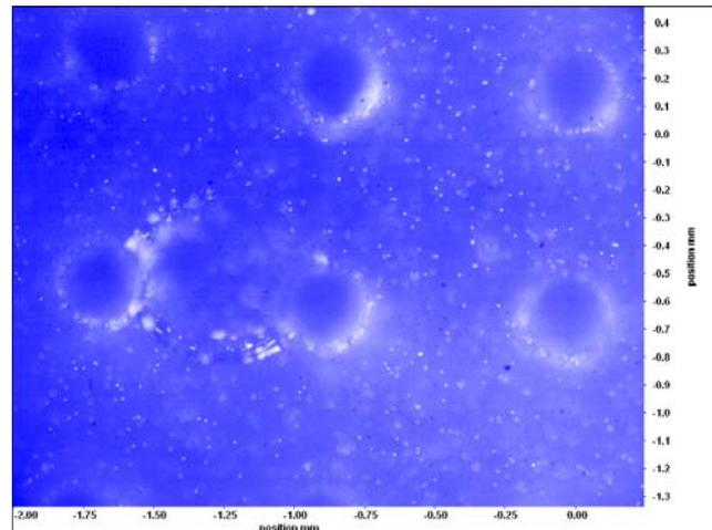
Fig.12 Optical view of air bubble trapped between fibres
