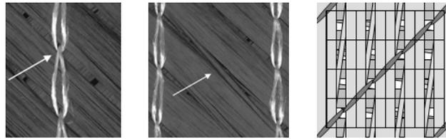
*Fig. 1. Top view of a biaxial NCF showing a) the thread and b) the crossings. c) Typical distribution of the different features from the stitching process in a biaxial NCF and its unit cell distribution.*
