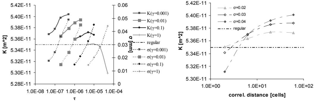
Fig. 4. The influence of a) the Monte Carlo parameters  $\tau$  (bottom axis),  $\gamma$  (in legend) and b) the correlation distance on the global permeability for different standard deviations for a network structure including the thread and the crossings as in Fig. 1c.
