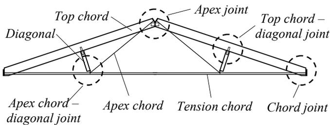
Fig. 5 The components of a pre-stressed tied rafter.
