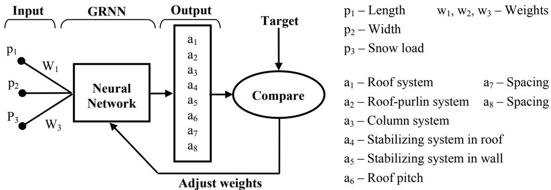
Fig. 4 The basic functionality of a neural network and the inputs/outputs used for the EFS.
