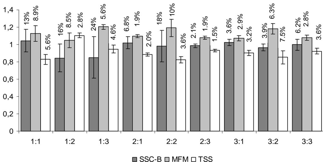
**Figure 1.** The average of five sub-samples for each individual method divided by the average of the sub-samples for all the methods (15 samples in total). CV (%) was calculated for each individual method, for rain events 1-3 (rain event : sample).
