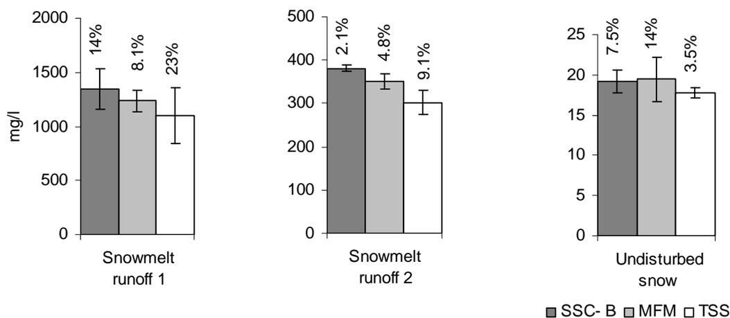
**Figure 2.** Measured mean solids concentrations (mg/l) and CVs (%)
