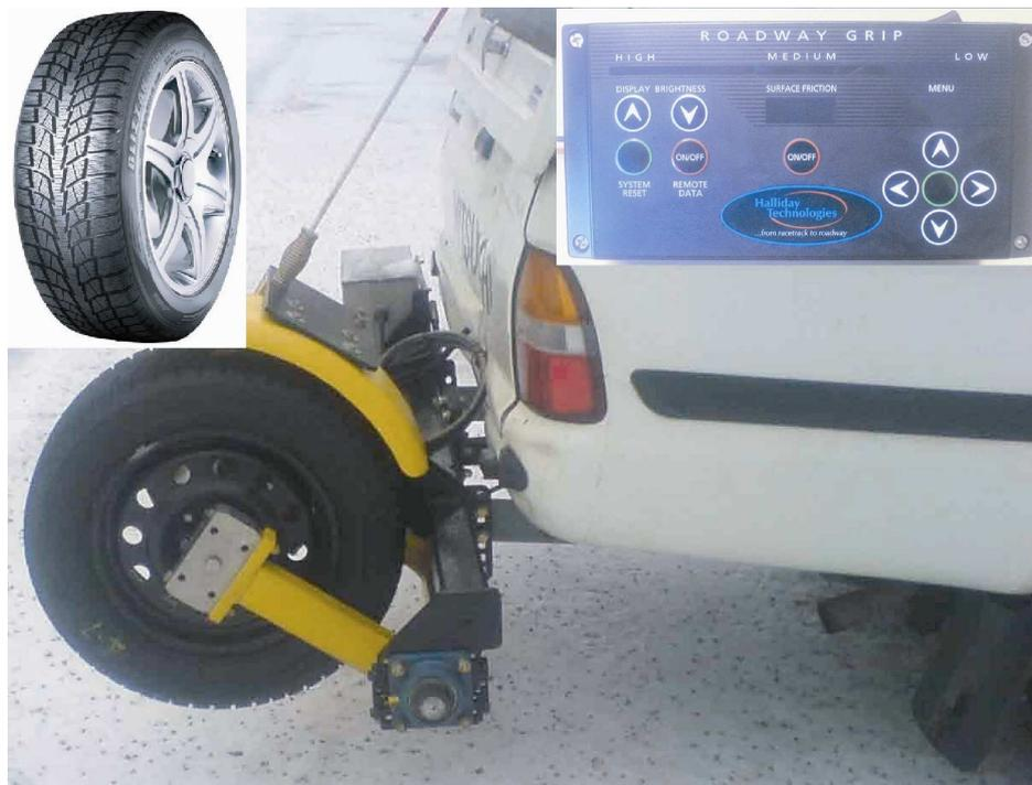
**FIGURE 1** RT3 tow hitch model mounted on Mitsubishi L200, in upper left corner tire pattern and in upper right corner display unit.
