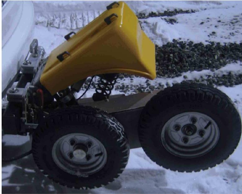
**FIGURE 2 TWO device with type 523 Trelleborg friction tires.**
