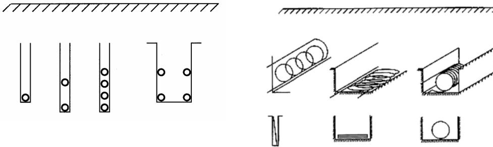
Figure 2. Different horizontal pipe systems for extraction of heat and cold from the ground.
