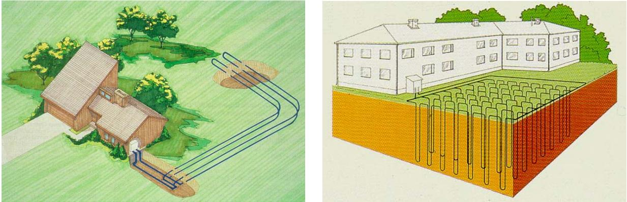
Figure 1. Examples of horizontal and vertical ground coupled pipe systems for space heating and cooling. Left shows a system with two pipes in each ditch.
