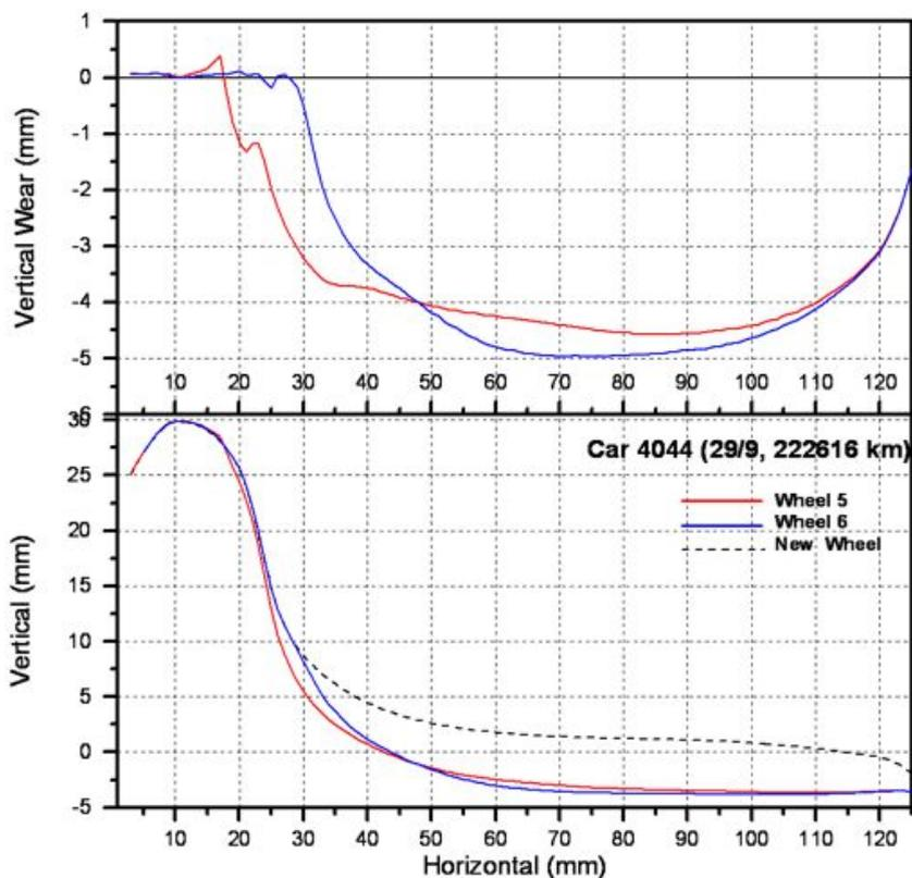
Figure 16. Vertical wear illustration of axle 3 in car 4044
