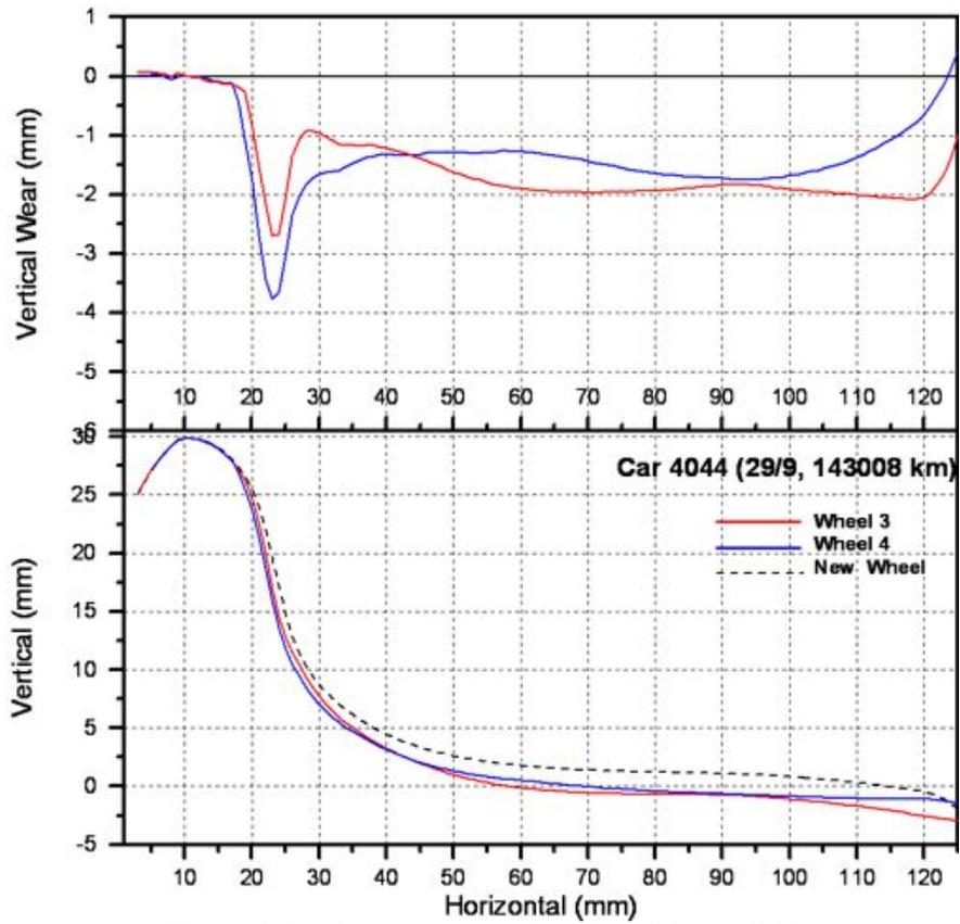
Figure 10. Vertical wear calculation of axle 2 in car 4044
