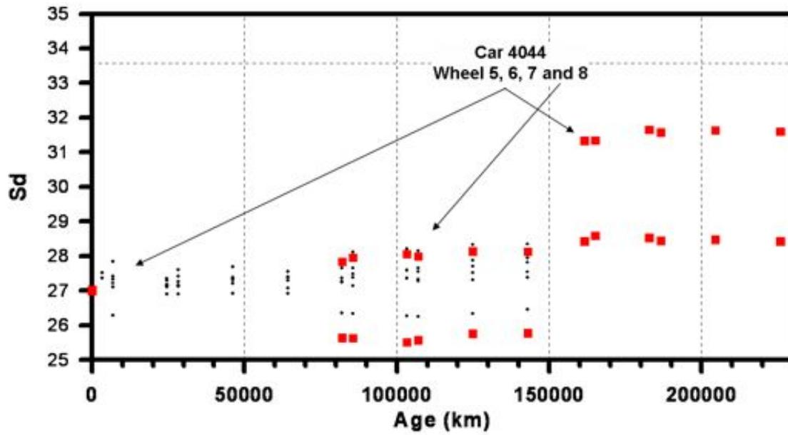
Figure 11. Flange thickness ( $S_d$ ) versus Age (km)
