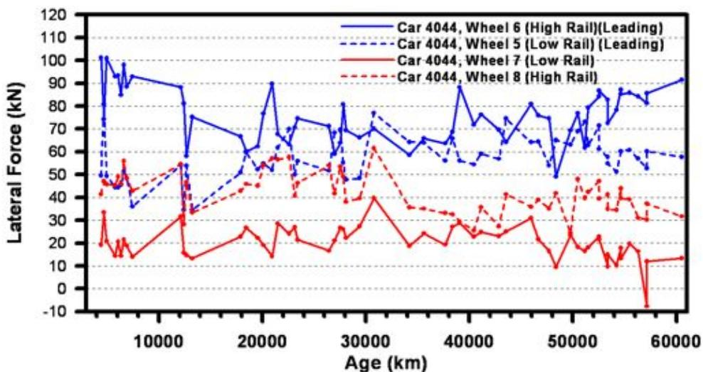
Figure 14. Lateral force (kN) versus Age (km) for a full bogie
