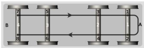
Figure 3. Measurement scheme and designation of wheels and axles.
