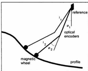
Figure 6. MiniProf™ measuring principle [4]
