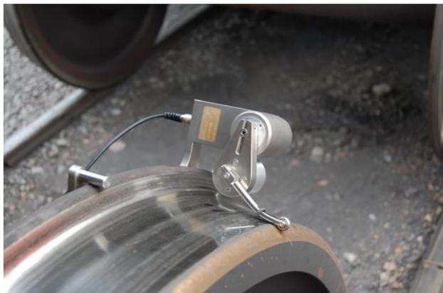
Figure 7. Wheel profile measurement by MiniProf™
