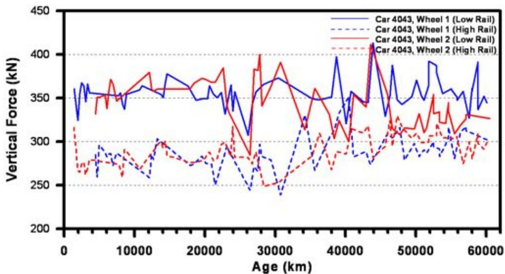
Figure 13. Vertical force (kN) versus Age (km)
